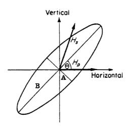
By measuring the angle from the horizontal to the longaxis of the ellipse  $(\theta)$ , a conductor is located when this tilt angle is zero.
