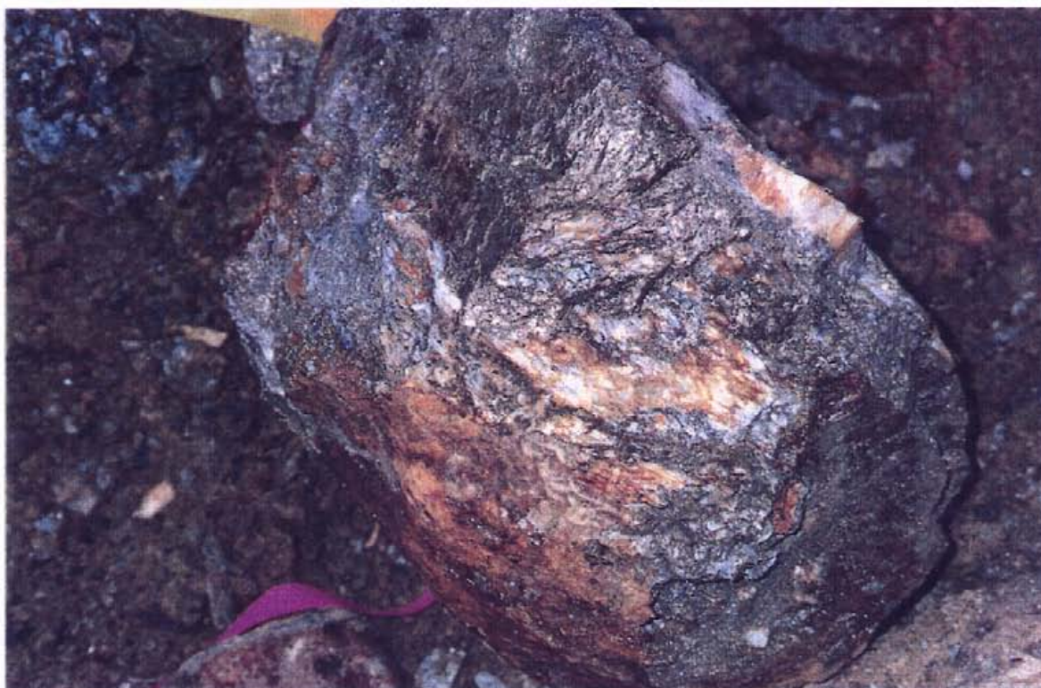
Sample 95882 chalcopyrite + sphalerite quartz vein mineralization
