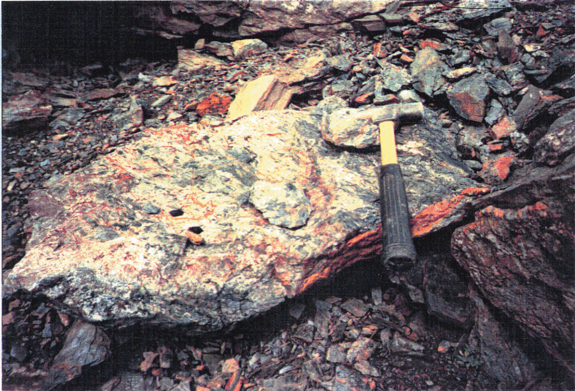
Photo 2. Mineralized Quartz-Carbonate Veins in Phyllite (Trench 9).
