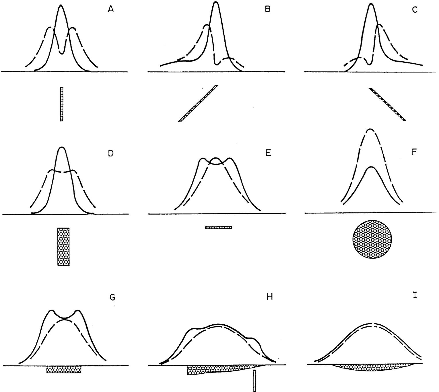
conductor becomes relatively significant and complete null coupling with the coplanar coils is no longer possible.(Profile D) As a result, the apparent minimum of the coplanar response over the conductor diminishes with increasing thickness, and in the limiting case of a fully 3 dimensional body or a horizontal layer or half-space, the minimum disappears completely.
