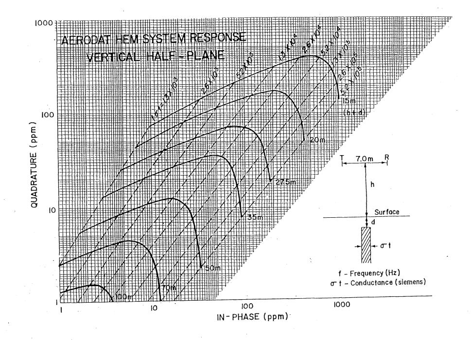
and/or strike and adjacent bodies and overburden may have modified the response. In general the conductance estimate is less affected by these limitations than is the depth estimate, but both should be considered as relative rather than absolute guides to the anomaly's properties.
