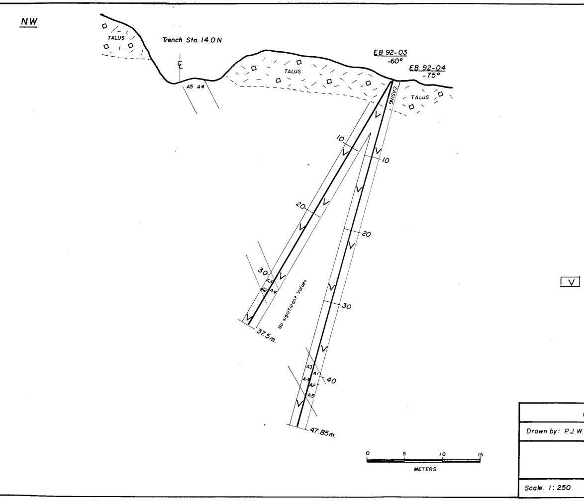
SE GEOLOGICAL BRANCH ASSESSMENT REPORT 22,820 LEGEND TAKLA METAVOLCANICS Dark green in color ALTERATION A! CHLORITE - EPIDOTE A2 PYRITIC A3 BLEACHED A4 SILICIFIED AS BRECCIATED CANASIL RESOURCES INC. Date: January 1993 EB ZONE D.D.H. EB 92 - 03 and EB92-04 BRENDA PROPERTY Toodoggone Area B. C. Draw. No. 92-10
