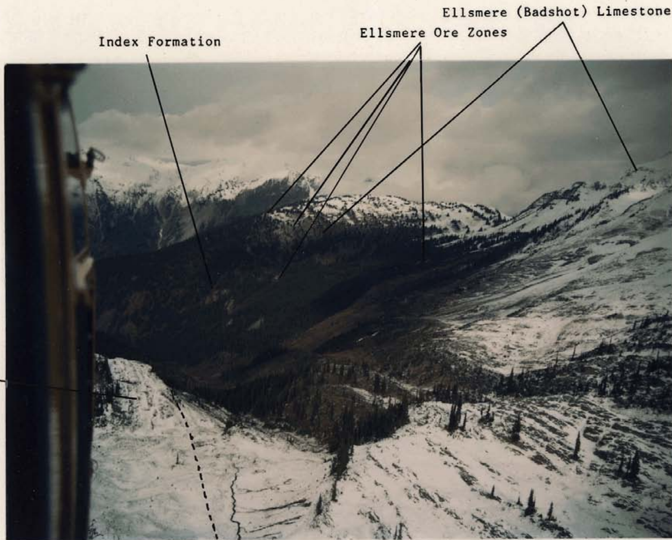
Fig. 3 Oblique photo looking north showing the Horne Ledge Limestone (part of Index Formation), Index Formation, and the Ellsmere Limestone (Badshot Formation). The Horne Ledge and Ellsmere limestones are hosts to several Mississippi-Valley-type massive sulfides. The main Ellsmere ore zone was traced for more than 1280 meters (4200 feet) along strike in 1992. Total strike length of the Ellsmere zone is 2600 meters (8567 feet).
