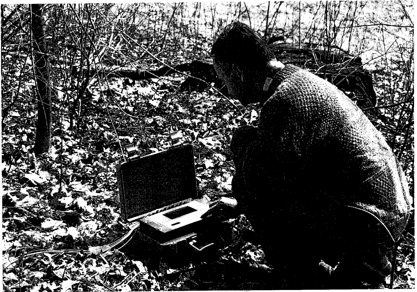
The IPR-12 Receiver measures spectral IP signals from eight dipoles simultaneously then records measured and calculated parameters in memory.
