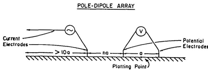
The dipole length and reading interval was chosen to be 50 metres for all survey lines. The lines were read to six separations which gives a theoretical depth penetration of 180 m (about 600 feet).
