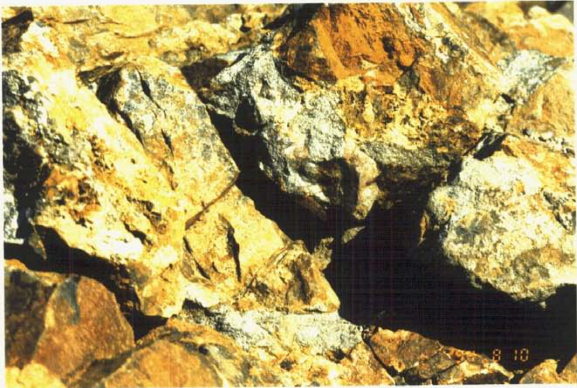
Photo 18: Area of intense sulfidization - Sample 70220. Veins and lenses of massive pyrite in silicified volcanics
