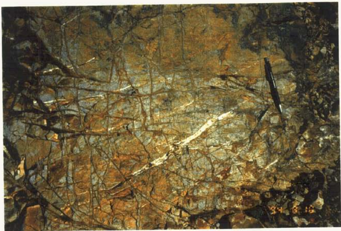
Photo 19: Stockworking of quartz & oxidized material in silicified volcanic
