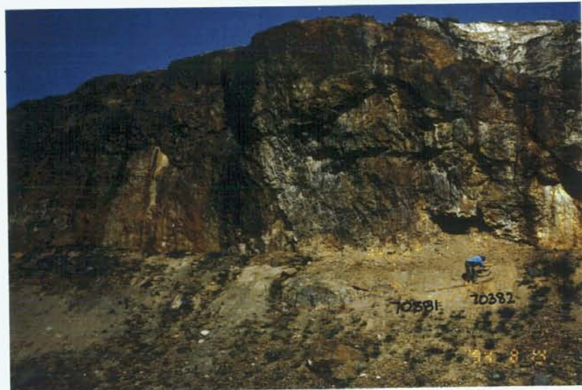
Talus channel sampling below jarosite/alunite alteration
