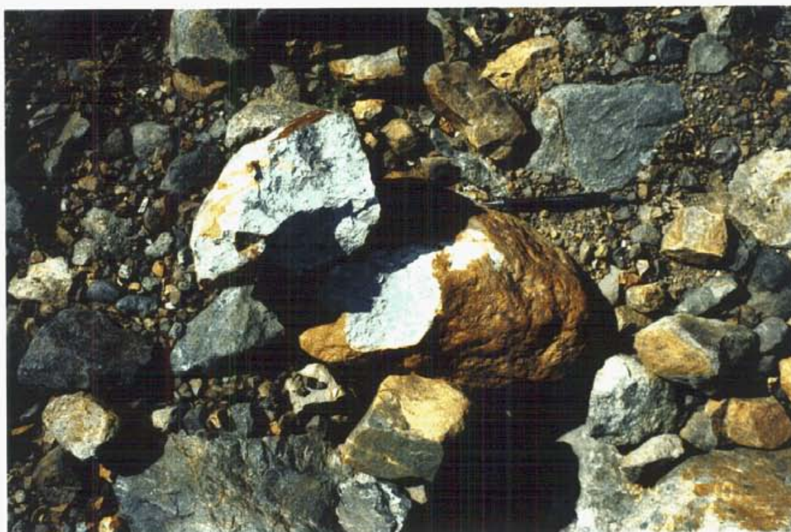
Photo 20: Massive sulfide float boulder - Sample 70230
