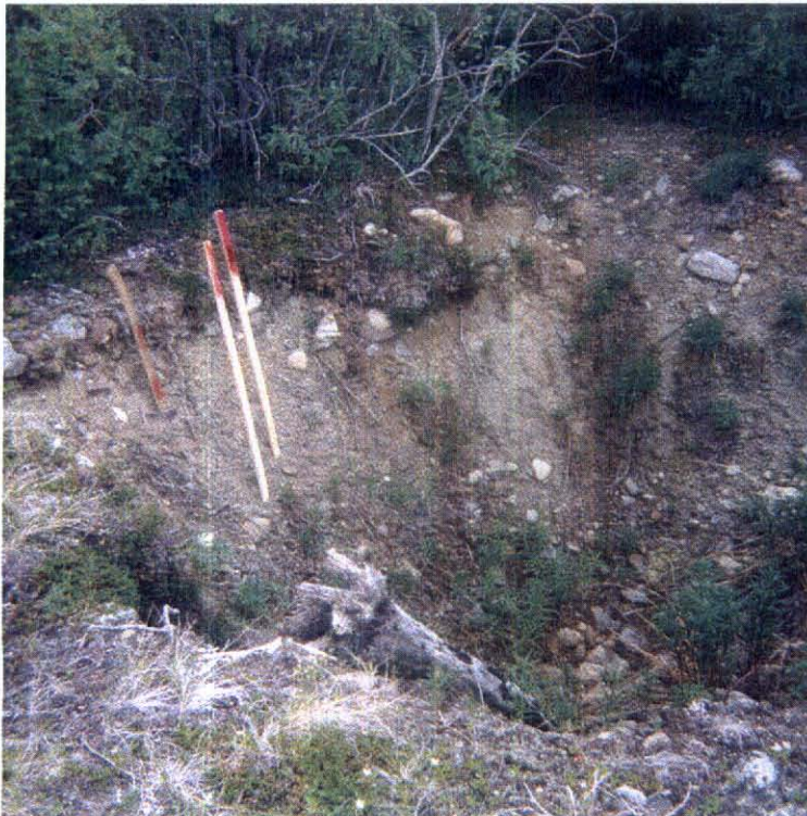
SINK HOLES FROM CAVED UNDERGROUND LOCATED APPROX. 100 METRES UPSTREAM FROM PORTAL
