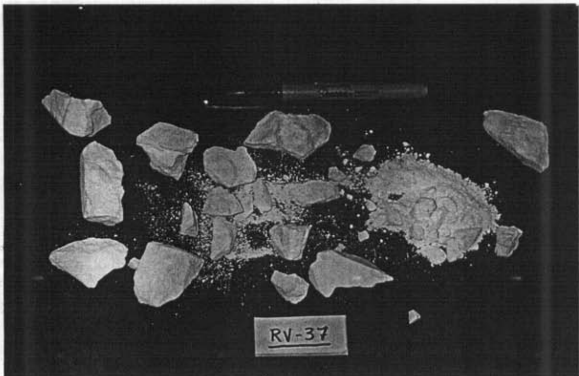
Fig. 4.4 Lime Pebbles and Fines after Decrepitation Testing of Sample RV-37.
