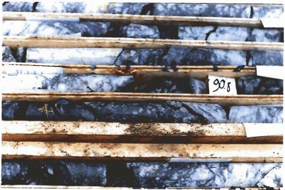
Photo 16 DDH 95-2; close up of mineralization in the vicinity of 90.8 metres. The bluish-grey shattered quartz (dendritic like) areas occur along the hangingwall and footwall section of a vein and contain the highest percentage of sulphides and gold values.
