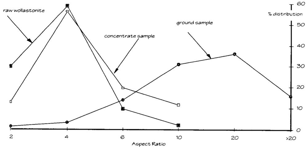
Figure 3-1: Aspect Ratios, progress from raw material to preliminary grind trials
