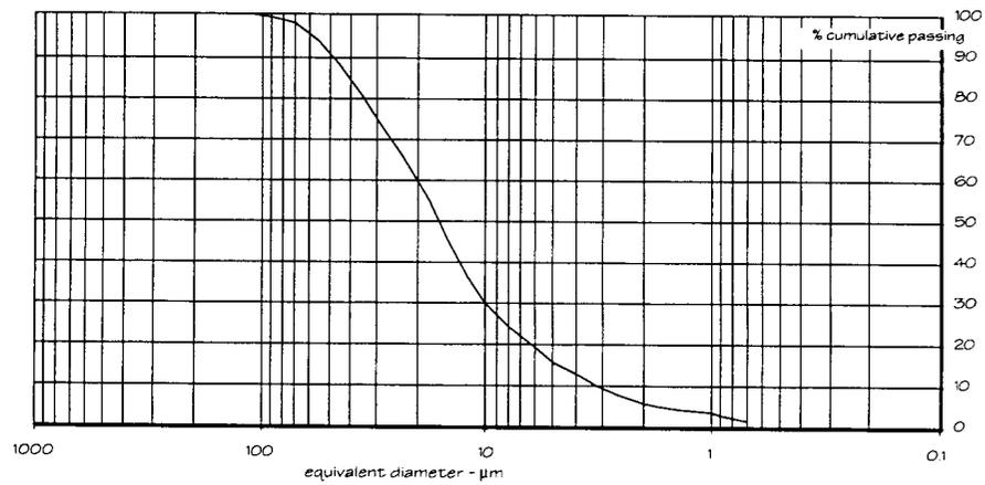
Figure 3-2: Particle size distribution for preliminary grind
