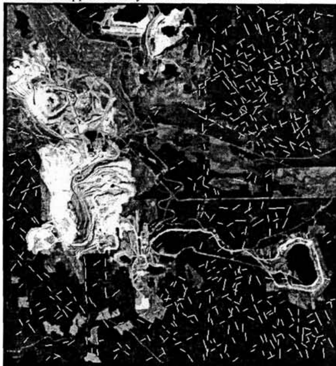
Image 5. Satellite image of Band 5 stretched showing individual linears. Window is approximately 12 kilometers east - west.
