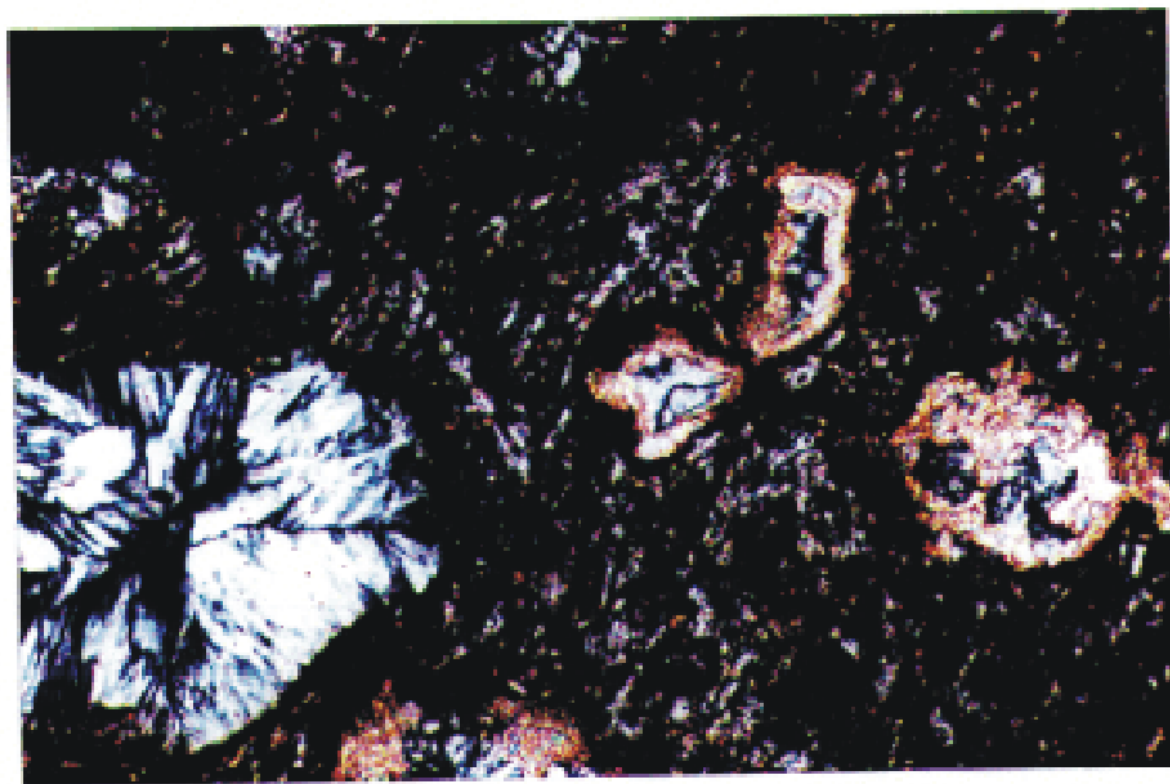
Micrograph 3: Amygdules are filled with radial chlorite and calcite (cross polarized light).
