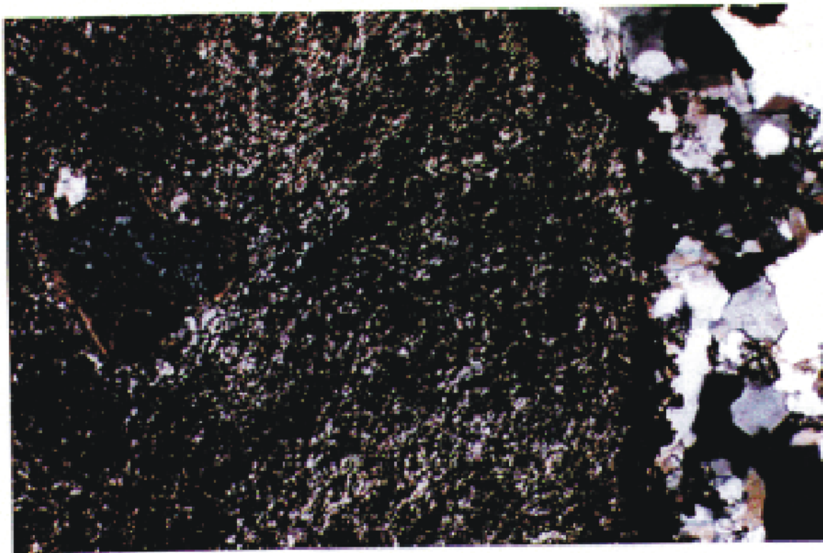
Micrograph 11: A vesicle filled with chlorite, calcite, quartz and pyrite. The matrix is composed with quartz microcrysts and sericite, cross-cut by a vein of quartz, calcite and pyrite (cross polarized light).
