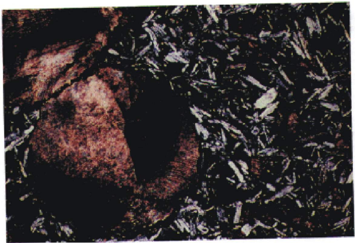
Micrograph 2: Amygdules and vesicles filled with calcite in a microlitic groundmass (cross polarized light).
