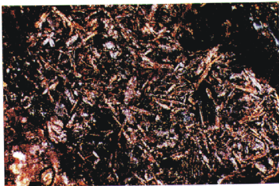
Micrograph 1: Microlites of plagioclase altered to calcite ( cross polarized light).
