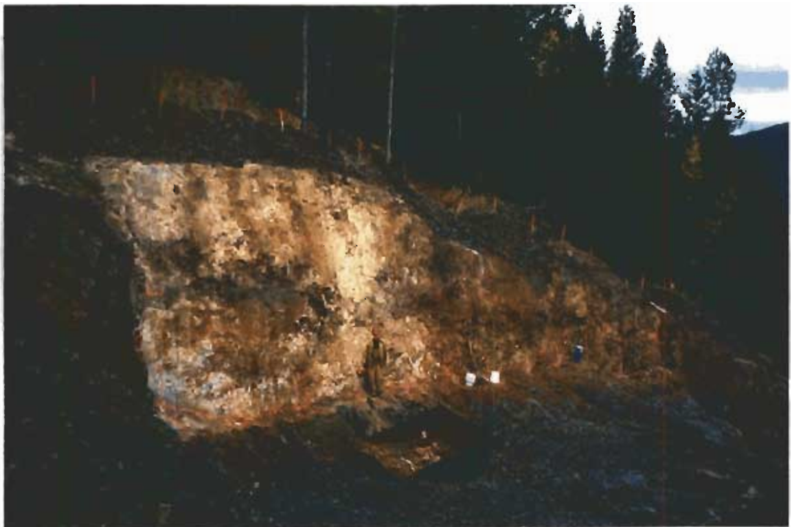
Photo # 2 - Vein stripped with floor ready to sample
