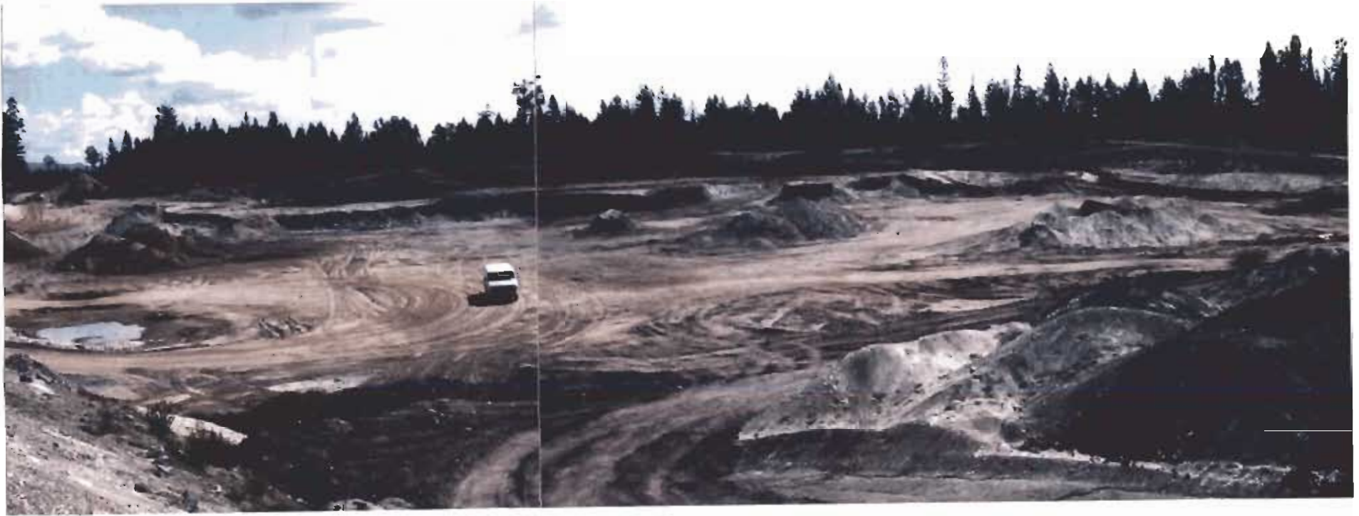
Plate 1: Red Lake Open Pit on August 26, 1995 viewed to the east from near Survey Station #1 on the waste pile, showing the ore pile, mounds of sedimentary breccia ( Mx ), each surrounded by waste, and the position of the bench front exposing the Upper D.E. Layer ( Mdu ). The locations of the other plates are shown.
