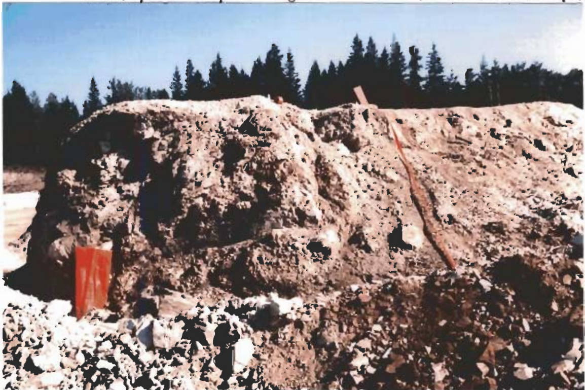
Plate 5: In Red Lake Open Pit at 118mE and 143mS, looking north at a sliver of sedimentary breccia ( Mx ) bounded by steep, north striking faults on the west (tape roll and plastic bag) and on the east (notebook and red tape).
