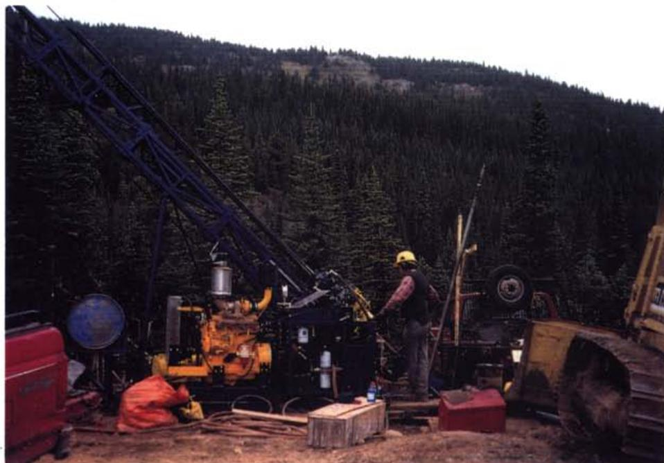
Figure 8.- Diamond drill working on DDH 98-3. Drill hole is being drilled at minus 45 degrees to the N. 65° E.
