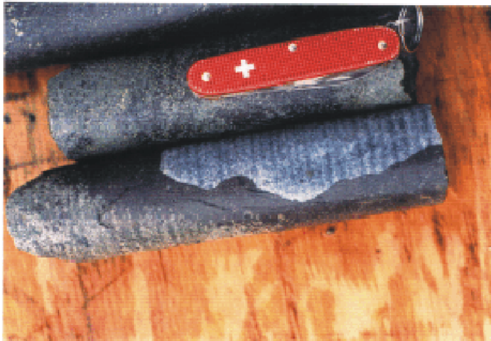
Figure 26: Close-up of upper contact of section in Fig. 25, showing concentration of sphalerite at marble contact. This is hand-sample scale version of zoning demonstrated overall by skarn-replacement transition zone.
