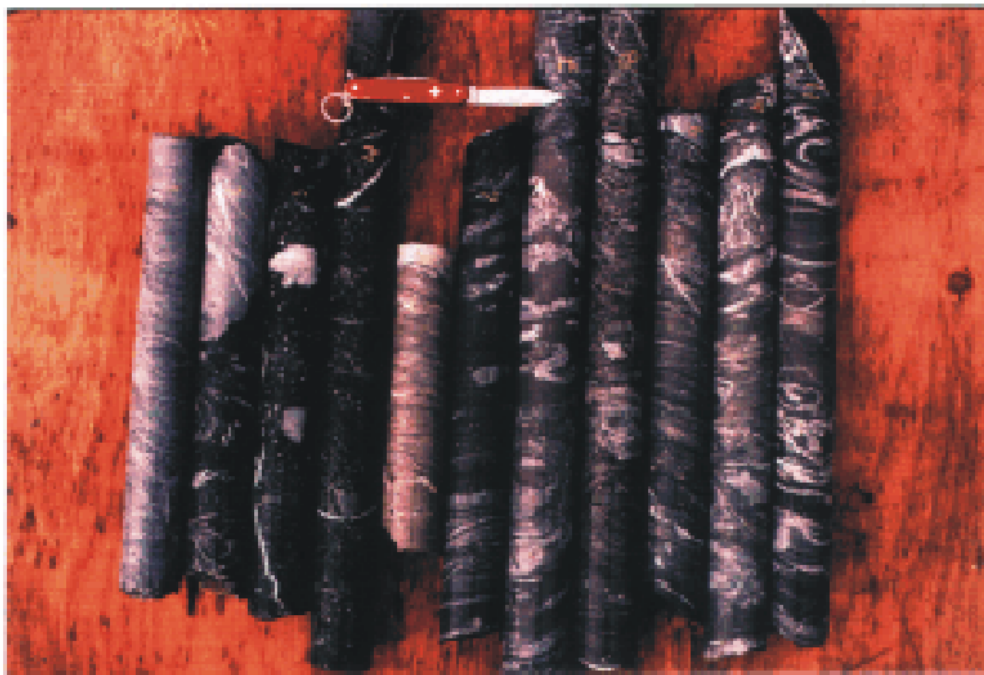
Figure 10: Core from LD99-16 [161 (top) 252 (bottom) meters depth, samples separated by about 10m each] showing transition from massive (grainflow?) limestone (1) to diminishing diameter limestone clasts in deformed argillite matrix (2-4) through a range of finely laminated argillite (5) with elongate and locally deformed limestone fragments (6-11).
