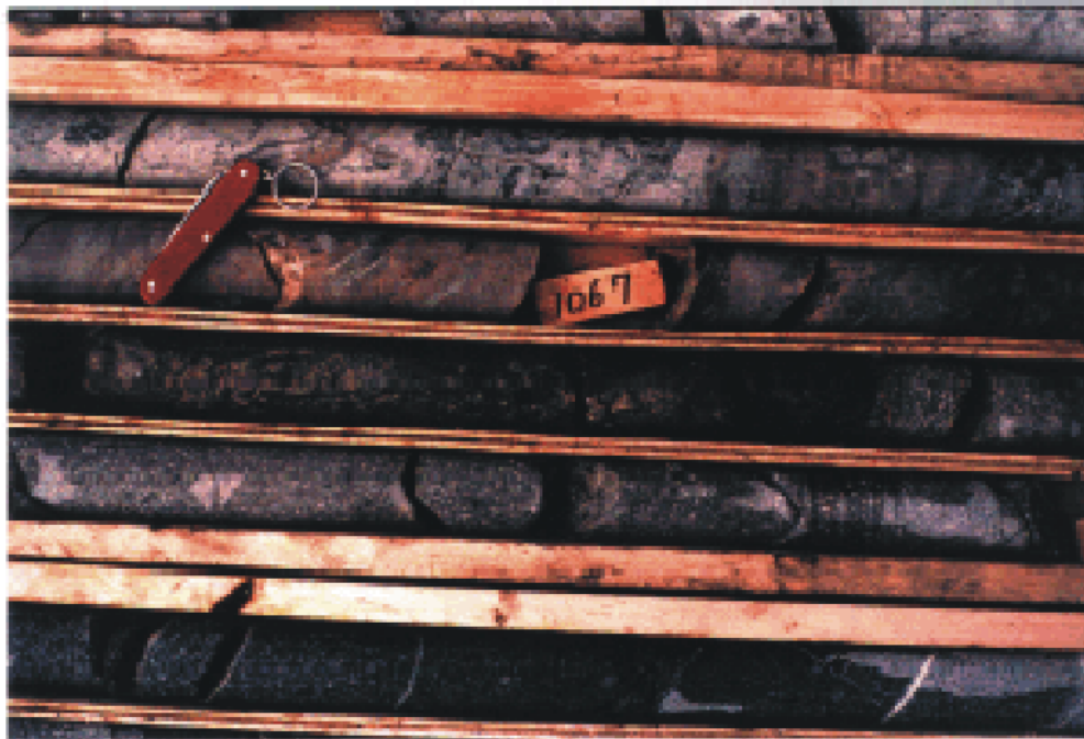
Figure 32: Close-up of retrograde skarn section from 339m depth in LD99-12, showing coarse magnetite patches with coarse chalcopyrite cutting across red-brown garnet stage (center) and replacing specularite (left center). This section (Sample 10380) ran 52.6 g/T Ag and 2.21% Cu.
