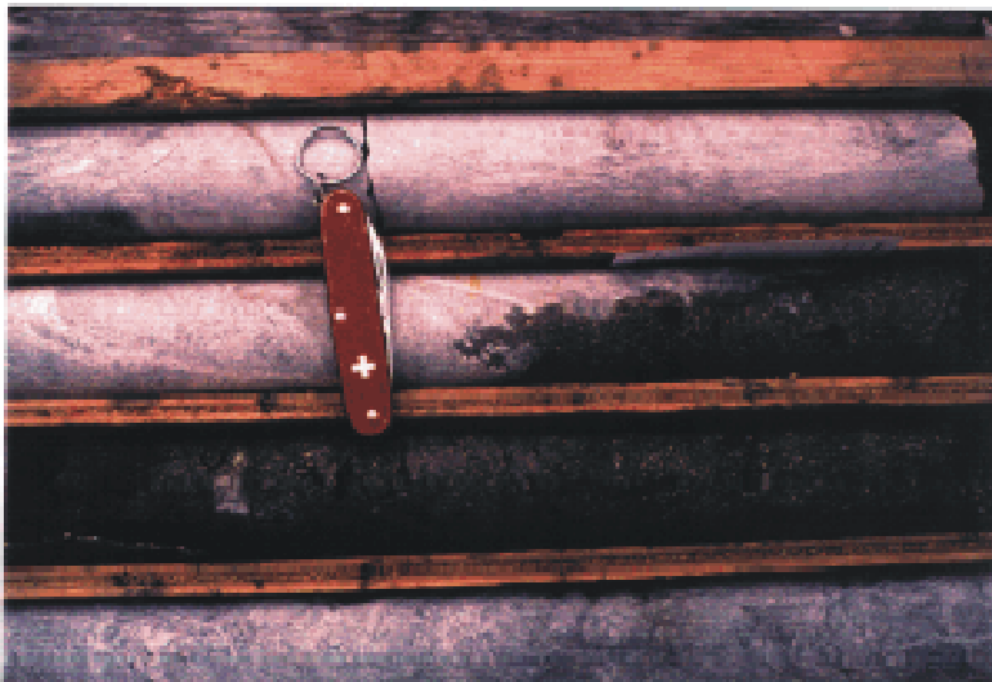
Figure 24: Close-up of contact between pyrrhotite and limestone. Note contrast between this coarse pyrrhotite and that seen in LD99-02 or LD99-16 (Figs. 9, 10, 13 ). Further note contrast between "invasion" of limestone by pyrrhotite and "clastic" contact in Fig. 14.
