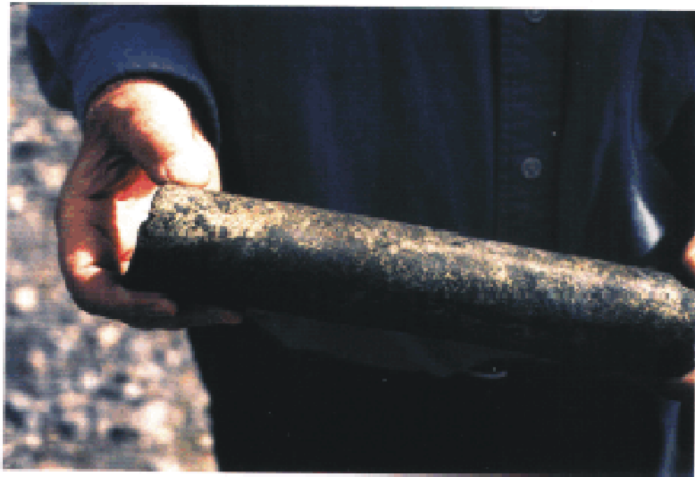
Figure 28: Close-up of chalcocopyrite-sphalerite-rich garnet skarn from 83m depth in LD99-17. Section ran (Sample 10413) 1.74 g/T Au, 42.8 g/T Ag, 1.8% Cu, and 7% Zn over 1.2m.
