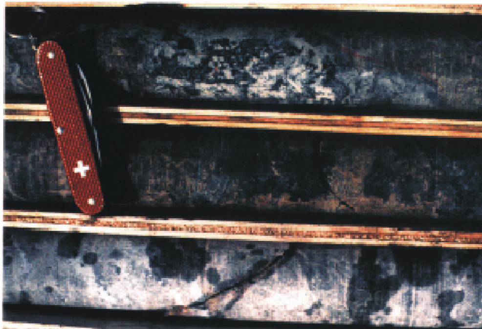
Figure 32: Close-up of retrograde skarn section from 339m depth in LD99-12, showing coarse magnetite patches with coarse chalcopyrite cutting across red-brown garnet stage (center) and replacing specularite (left center). This section (Sample 10380) ran 52.6 g/T Ag and 2.21% Cu.
