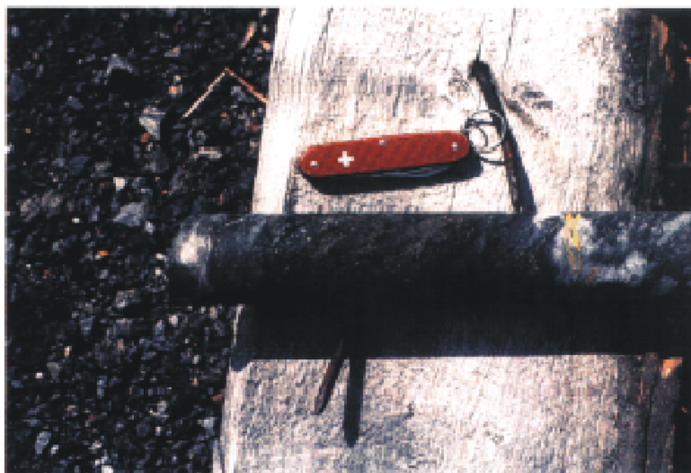
Figure 22: Close-up of 30 cm thick sphalerite-rich vein intersected in LD99-14 at 36m. Intercept (Sample 10388) ran .7 g/T Au, 134 g/T Ag, 0.6% Cu, 2.3% Pb, and 7% Zn.
