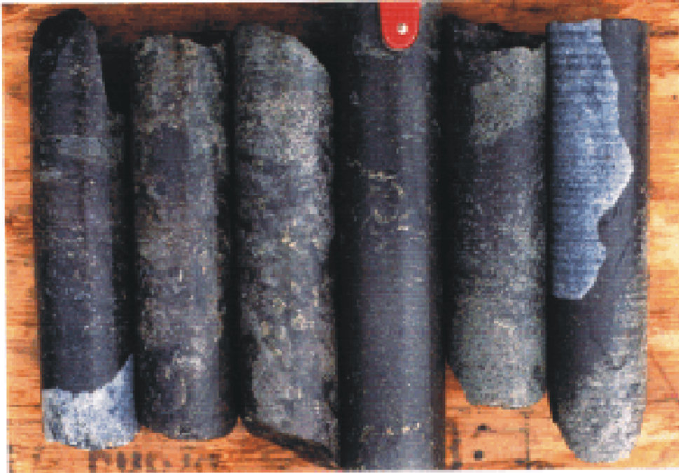
Figure 25: High-grade sphalerite-chalcopyrite-rich skarn from LD99-17 (77.5-83.5m, top to right), showing sharp contacts with limestone, sphalerite replacing skarn (greenish) and late chalcopyrite interstitial to sphalerite. Also note moderate retrograde hydration of skarn (cream-colored areas in sections 2 and 3 from the left). This section assayed 18.9% Zn, and 0.9% Cu.
