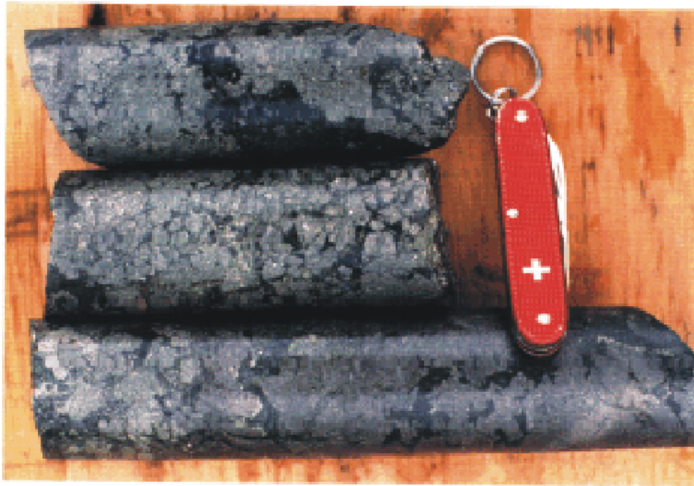
Figure 27: Close-up of core from 58m in LD99-17, showing massive pyrrhotite replaced by coarse-grained pyrite with interstitial chalcocopyrite.
