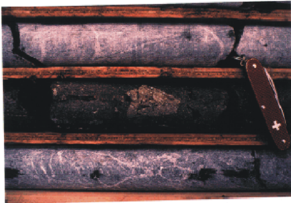
Figure 20: Finely banded pyrrotite from LD99-13 at 82m, showing near-conformity between limestone bedding and pyrrotite banding. Note coarse pyrite replacement of pyrrotite to left of knife.
