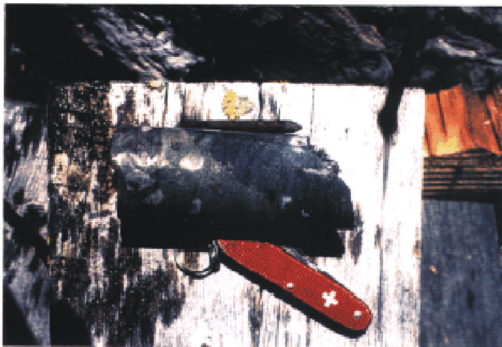
Figure 29: Core section from LD99-07, showing garnet skarn progressively replacing hornfels. Garnet is pervasive at top of section, and along narrow bands between very cherty layers. Note diagonal fractures with skarned margins that connect between skarned hornfels layers.
