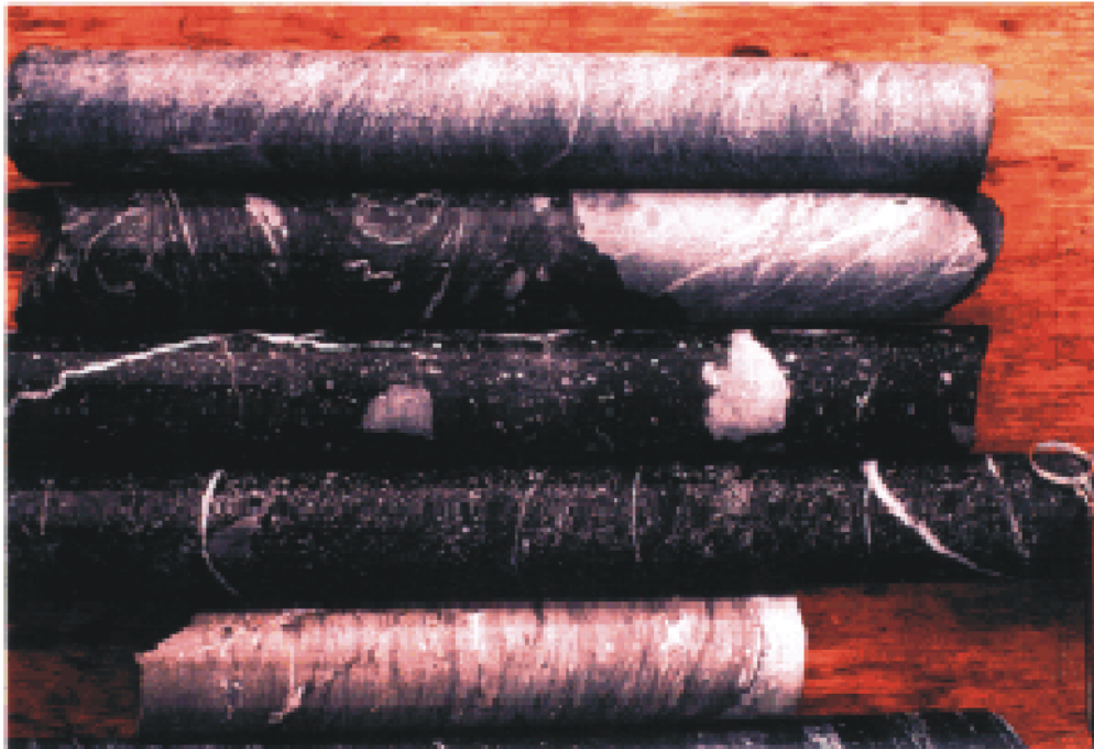
Figure 11: Close-up of core sections 1-5 from Fig. 10 [ samples separated by about 10m each] showing transition from massive (grainflow?) limestone (1) to diminishing diameter limestone clasts in deformed argillite matrix (2-4) to finely laminated argillite (5). This sequence appears to be a typical turbidite Bouma sequence; this indicates that the section is overturned.
