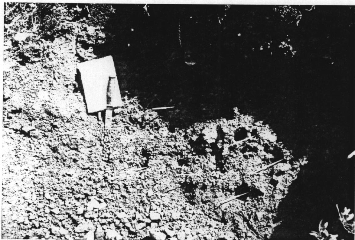
Fig. 4. Clast fabric analysis in basal till. Aluminum knitting needles placed in pebble casts parallel to the long axis of the pebbles and plunge.
