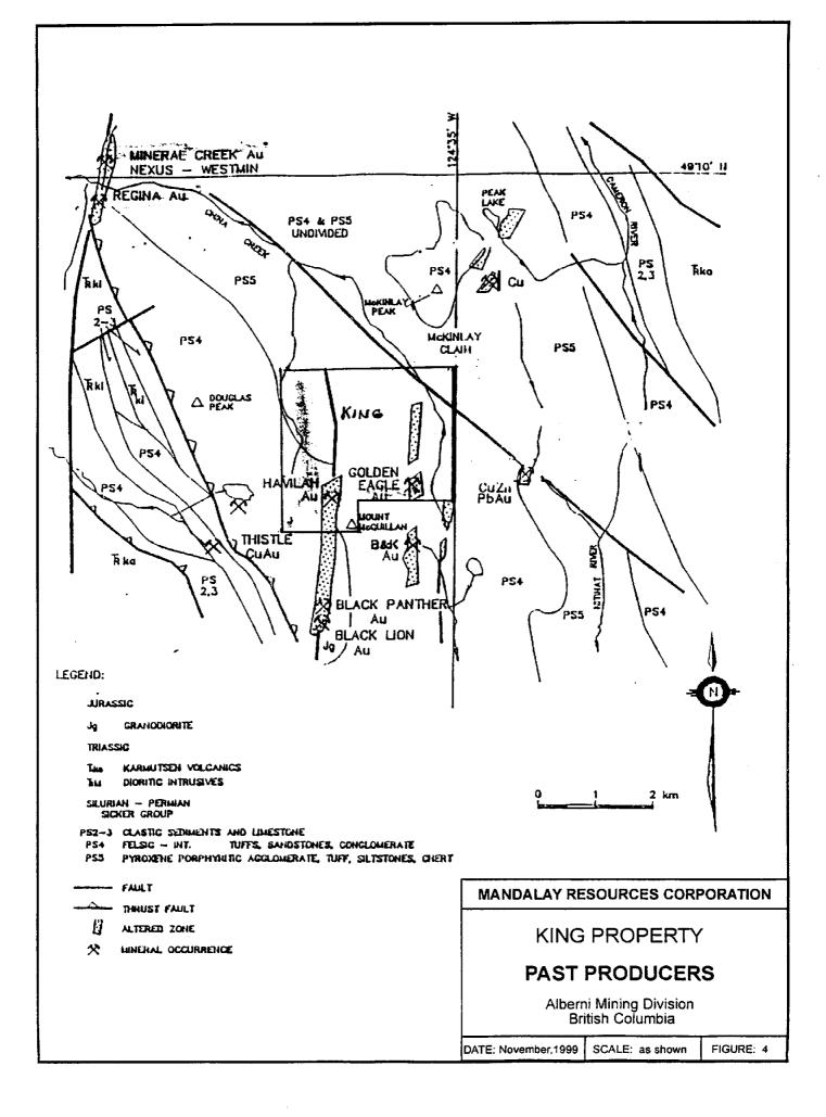
Extensive west-northwest trending faulting occurred during the Tertiary and is best illustrated by large displacements of Nanaimo Group sediments. The north trending Alberni Valley fault is traced over 45 miles and displaces a section of Karmutsen Formation approximately 5,000 feet (Muller and Carson, 1969).
