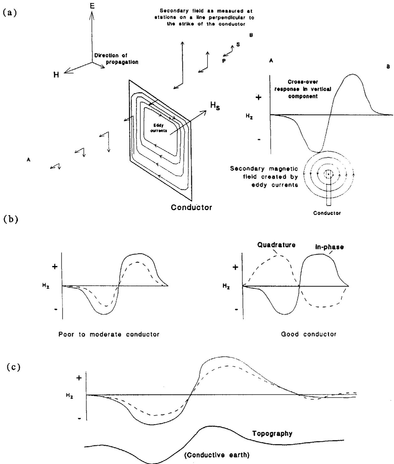
Figure VLF-2. VLF responses. (a) The horizontal magnetic flux from a VLF signal induces a secondary field in a conductor. This, together with the primary field, produces a cross-over response. (b) Quadrature sign can be determined by target conductance. (c) If the ground is conductive, topography can induce VLF responses similar to those expected from bedrock conductors.
