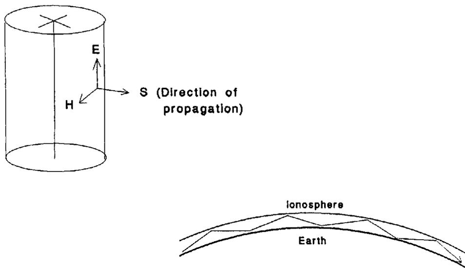
Figure VLF-1. VLF source fields and propagation. (a) Diagram showing Jim Creek, WA VLF transmitter (McNeill and Labson 1990). (b) Propagation of VLF field at a distance from the antenna. The VLF wave propagates between the earth's ionosphere and the surface with a vertical electrical field and horizontal magnetic field. At great distances the signal forms a plane wave.
