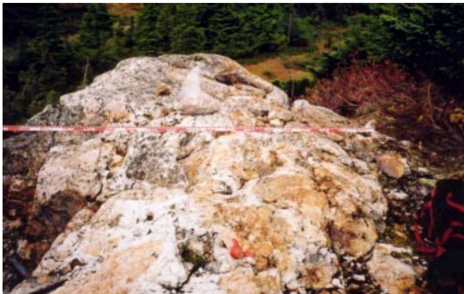
**Plate 6.** Zone of quartz-sulphide occurring at the intersection of a northwest trending structure and a main zone ledge (sample DHM-21: 12.6 g/t Au and 163 g/t Ag over 2.2 m).
