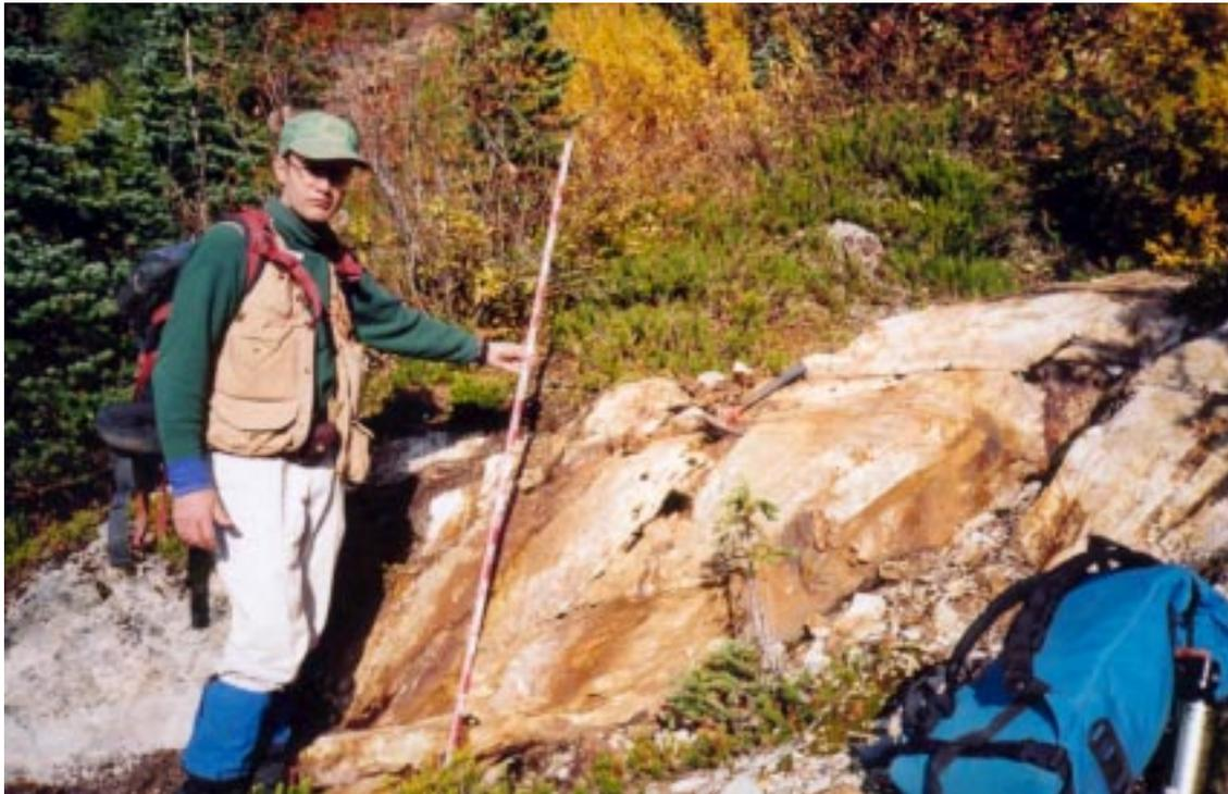
**Plate 4.** 2.8 meter (true thickness) exposure of main zone quartz-sulphide vein trending 260°/52°N, approximately 50 meters east of the Deer Horn Mine adit entrance. Site of sample DHM-1 (16.8 g/t Au, 605 g/t Ag over 2.8 m true width).
