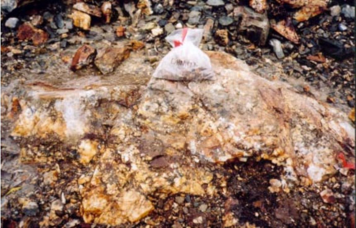
**Plate 7.** Northwest trending sulphide rich quartz vein, with sample DHM-23 sample bag for scale (DHM-23: 98.6 g/t Au, 2062 g/t Ag over 2.0 m).
