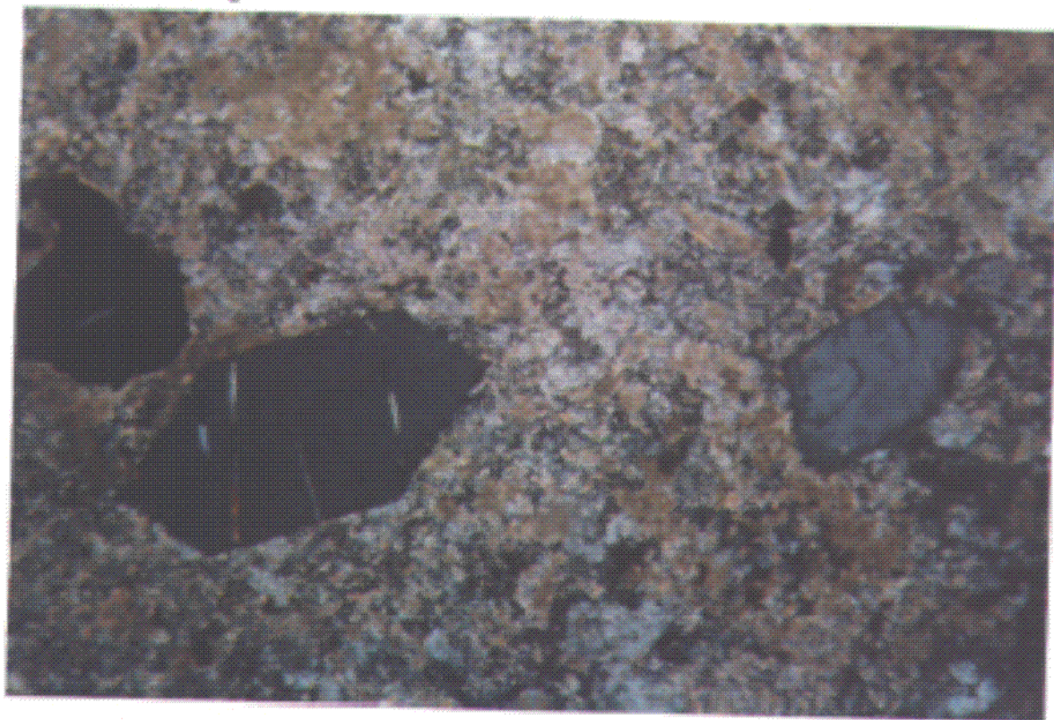
Above: R.04A. CP Light. Quartz Porphyry with corroded phenocryst (centre). Note feldspar phenocrysts pseudomorphed by fine sericite-carbonate. Fine grained aphanitic groundmass with quartz, feldspar, sericite, patchy carbonate. Below: R.06. CP Light. Euhedral weakly fractured K.feldspar phenocrysts in fine grained sericite carbonate altered groundmass.
