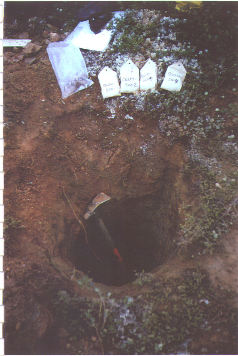
Photograph 7: Test Pit on Grid 2 at L 12+50 S/ 375E, shows collection of three soils from continuous horizons and also rock sample 126813
