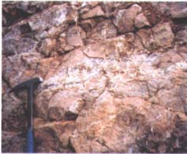
Plate 5 View of amethystine quartz breccia veining hosted within silicified massive trachyandesite in the upper pit of the AGB zone.
