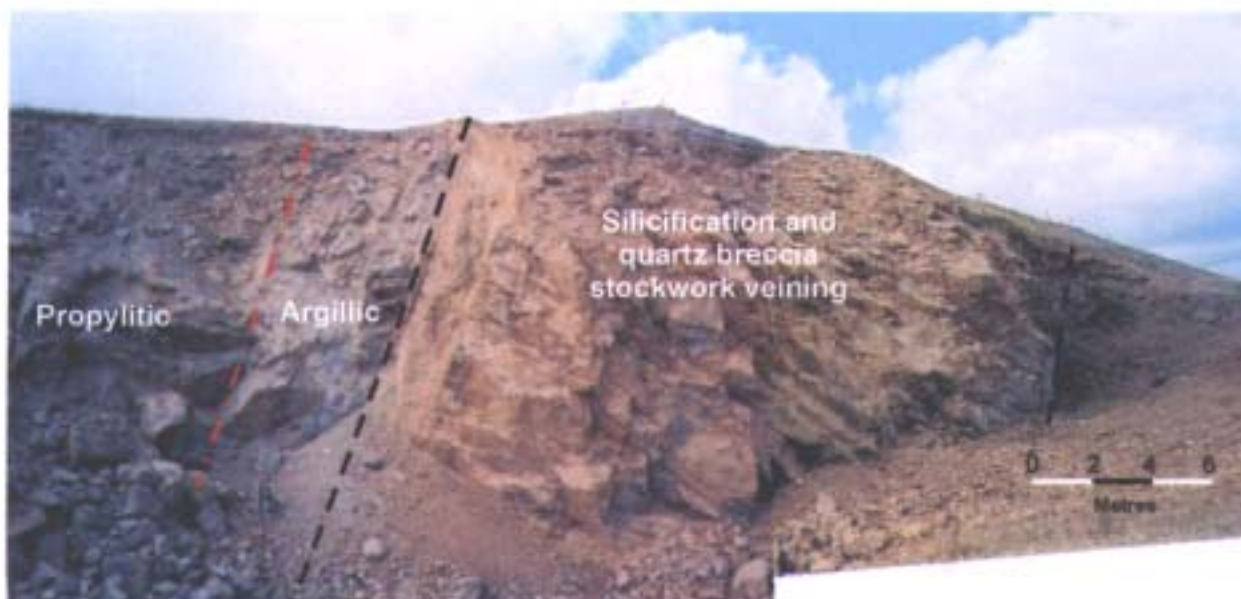
Plate 4 View to the north of the lower pit on the AGB zone showing the sharp, faulted contacts between zones of intense silicification and quartz breccia stockwork veining and argillic alteration.
