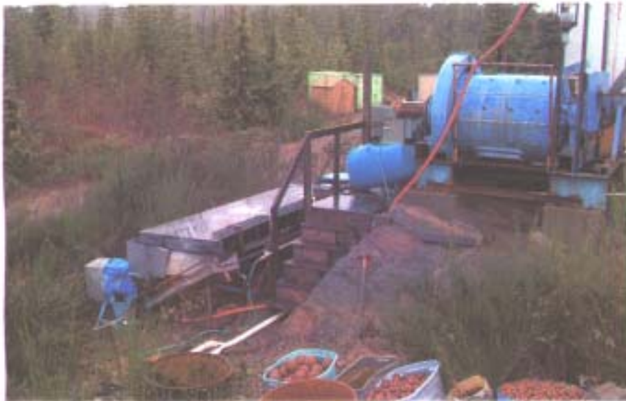
November 20, 2001 - Valentine Mountain Project - MINFILE 092B108 - gravity table below larger mill
