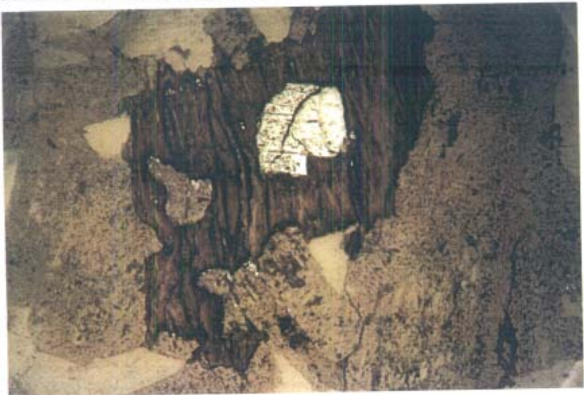
Above: PP. Light: Sample GN 97-64 PS 2B. Disseminated crystalline, orange-brown goethite in vein quartz. Below: Reflected Light Sample OXT-1. Specularite hematite pseudomorph after magnetite? enclosed in chloritic altered biotite (upper centre).
