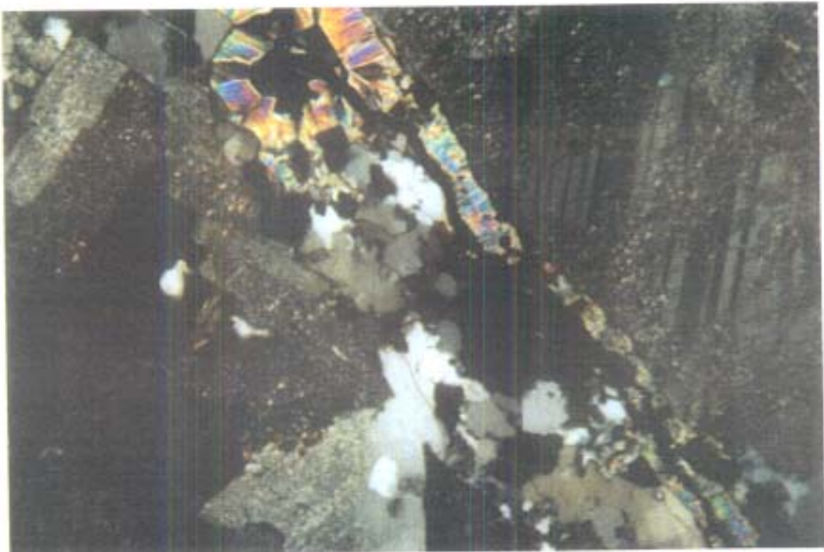
CP Light. Above: Sample GN 97-58 PS 1. Narrow penetrative quartz veinlets with fine oxides, no wallrock alteration. White mica-clay altered tabular plagioclase, interstitial fine quartz. Below: Sample OXT-3. Prismatic laumontite (zeolite) veinlets (pinks-blue) cutting earlier quartz vein (diagonal)
