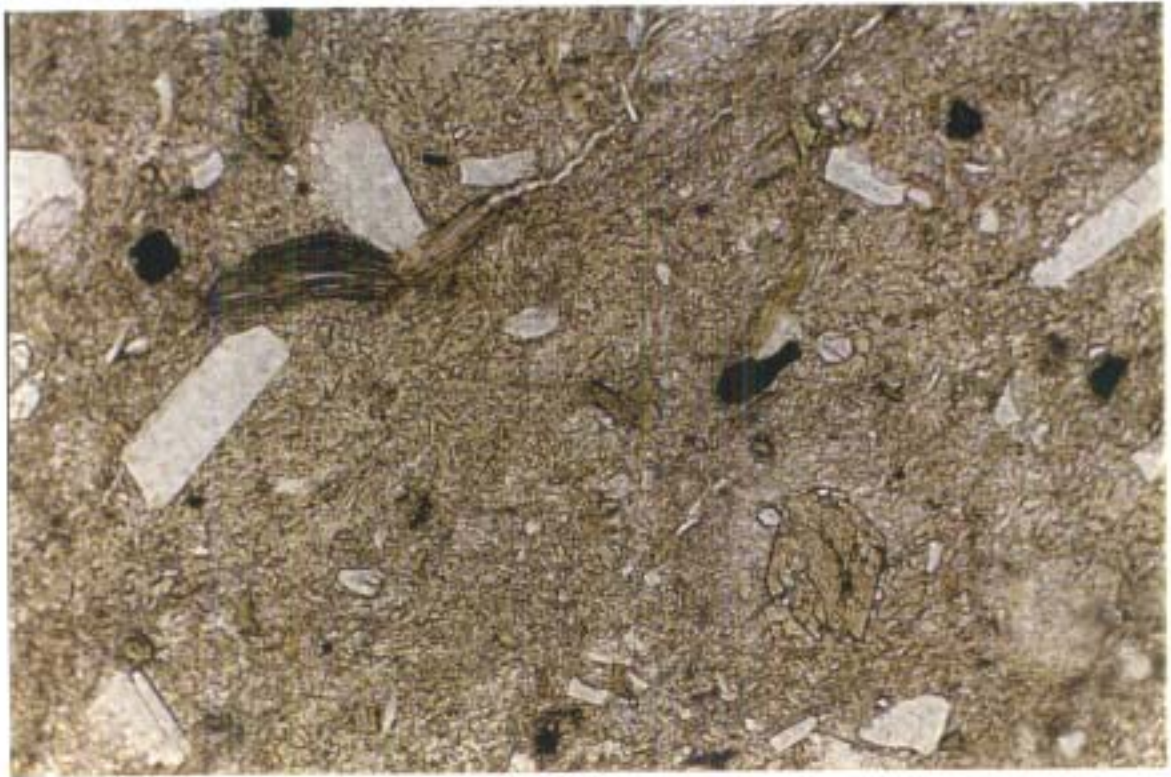
Photo 3 Photomicrograph of zeolitized dacitic crystal vitric tuff (sample Man-10b) (field 2\frac{1}{2} \times 4 mm)
