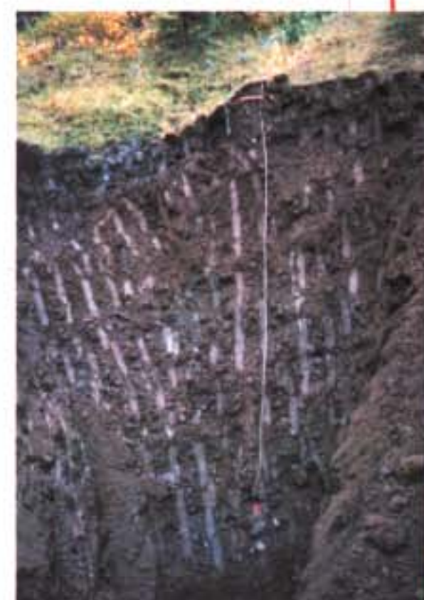
Test Pit PVT02-16 showing quality of glacial till.
