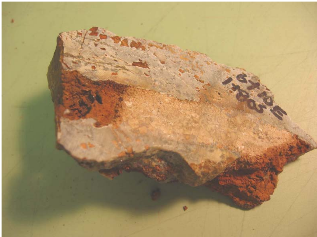
Photo 4 Felsic intrusive float cut by carbonate-quartz vein (Hook Lake Grid). Sample 931729 assayed 20.7 g/tonne Au.
