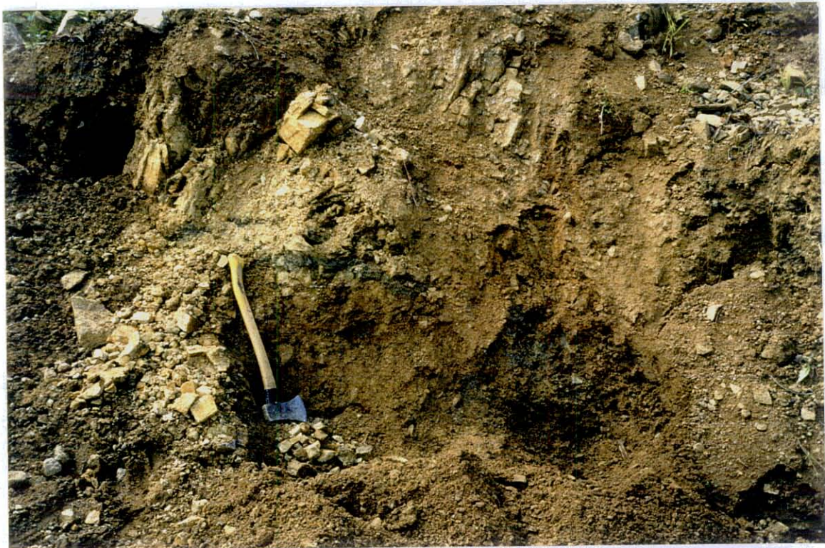
MEGATON: WEST WALL TRENCH No. 2, LANDING ZONE SHOWING FLAT DIPPING, MALACHITE-STAINED QV ZONE. SAMPLE NO. 02MT-6
