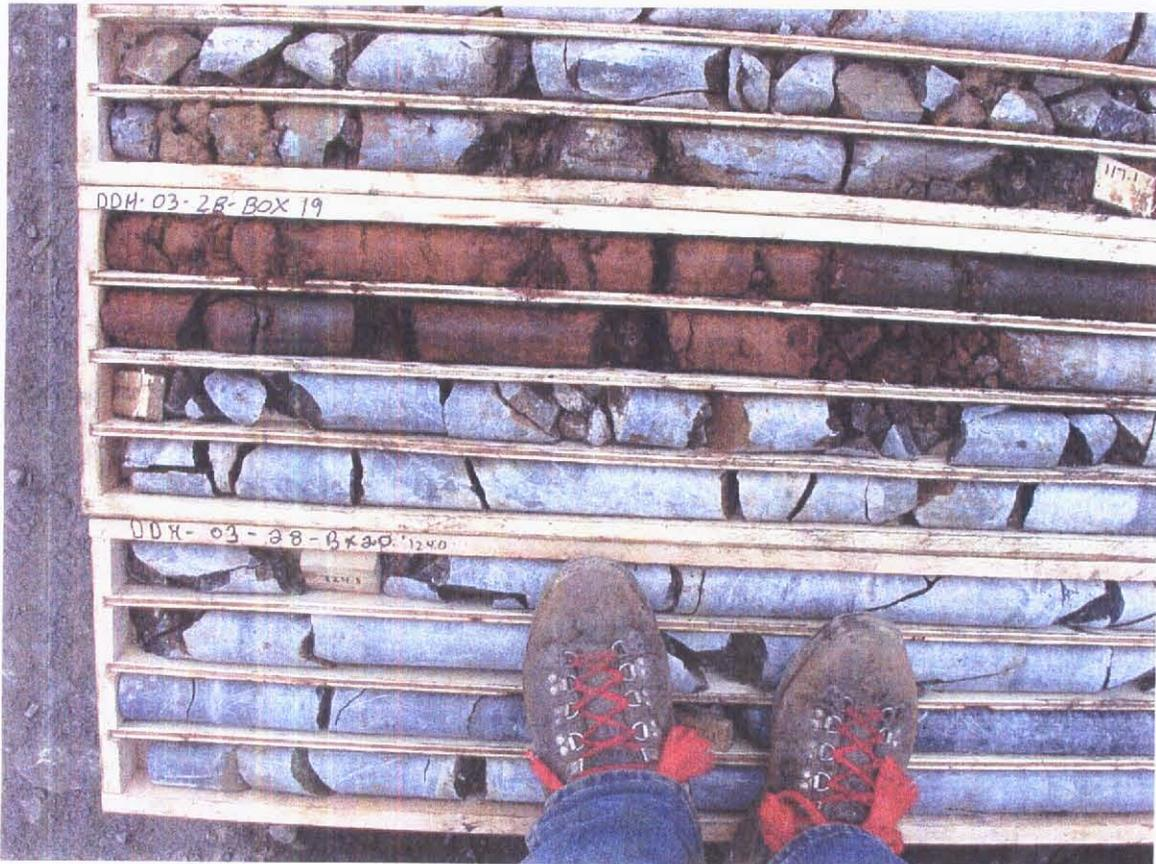
**Plate 5. Number 3 Zone Oxidized Mantos, DDH 3 – 28 @ 117 – 120.2 m.** The abrupt onset of the mineralized zone is clearly noted in this interval. Also of significance is the relatively competent nature of both the footwall and hangingwall contacts on this mineralized zone.
