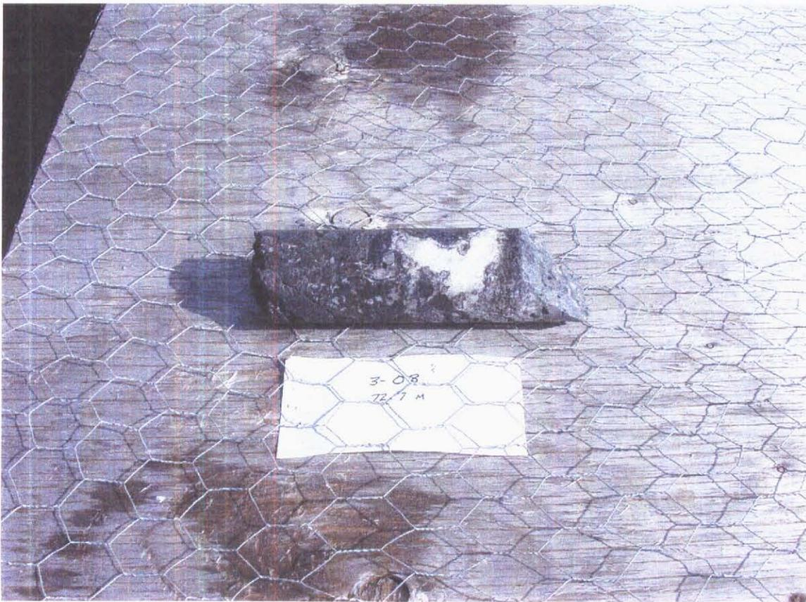
**Plate 1. High sulphide replacement vein DDH 3 – 08 at 72.7 m.** The white gangue mineral is calcite which exhibits moderate to weak banding. The intersection carried 1.2 g/t Au, and 458 g/t Ag over 5.5 m (73.8 – 79.3 m).
