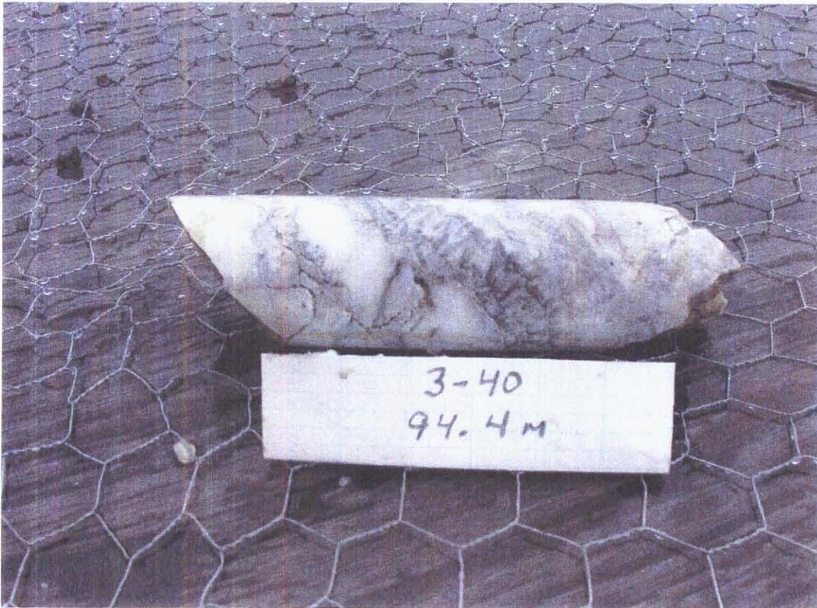
**Plate 7. Banded calcite, low-sulphide, orogenic vein, DDH 3 – 40.** This large vein extends from 93.2 m to 95.4 m. The vein is not significantly geochemically anomalous in either base, precious metals or mercury mineralization.
