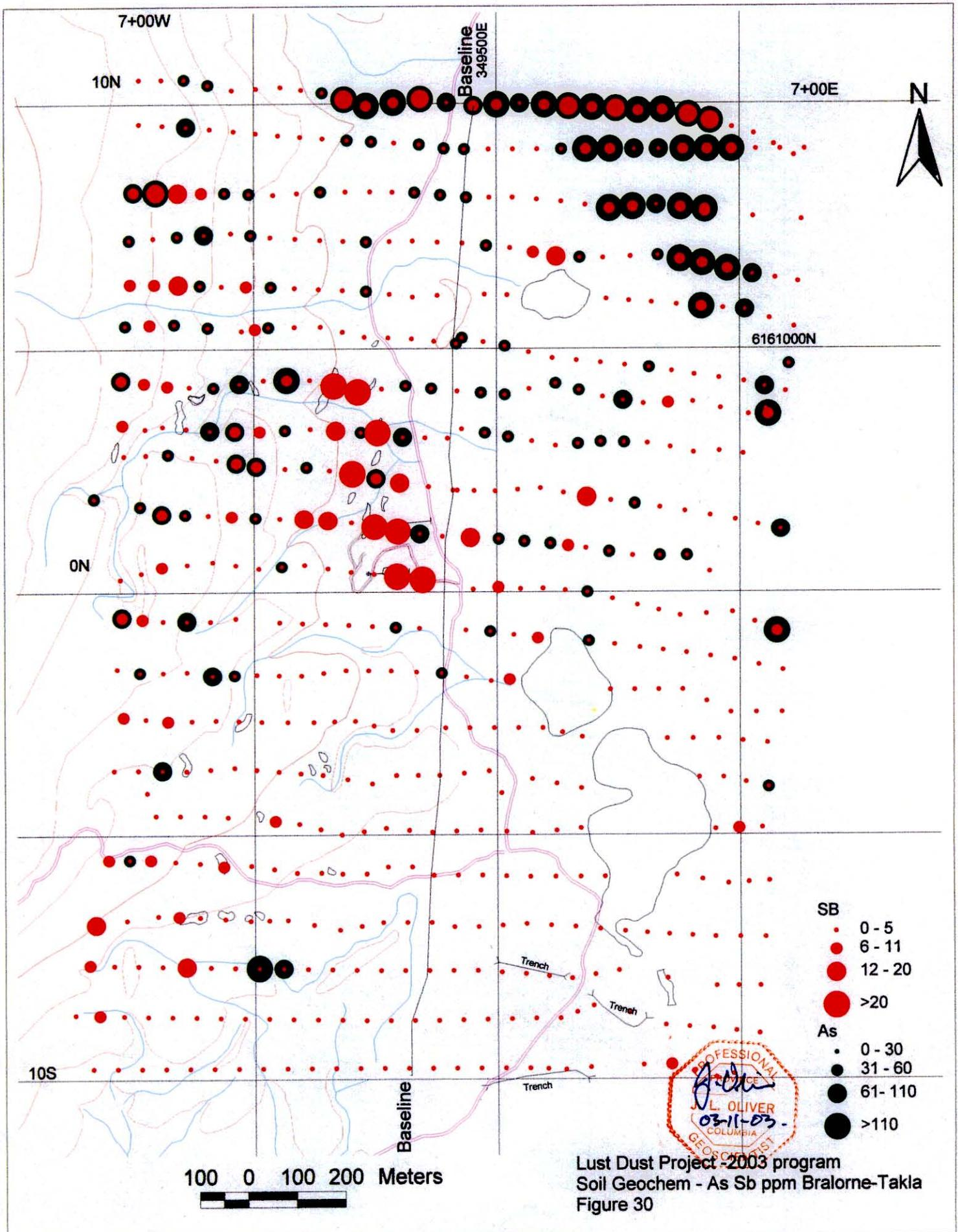
The three large trenches in the south central map area have no significant arsenic or antimony association. It is likely that these trenches have been placed largely on the strike relations of the main Balorne – Takla Mercury mine anomalies and related north-northwest trending structural zones.
