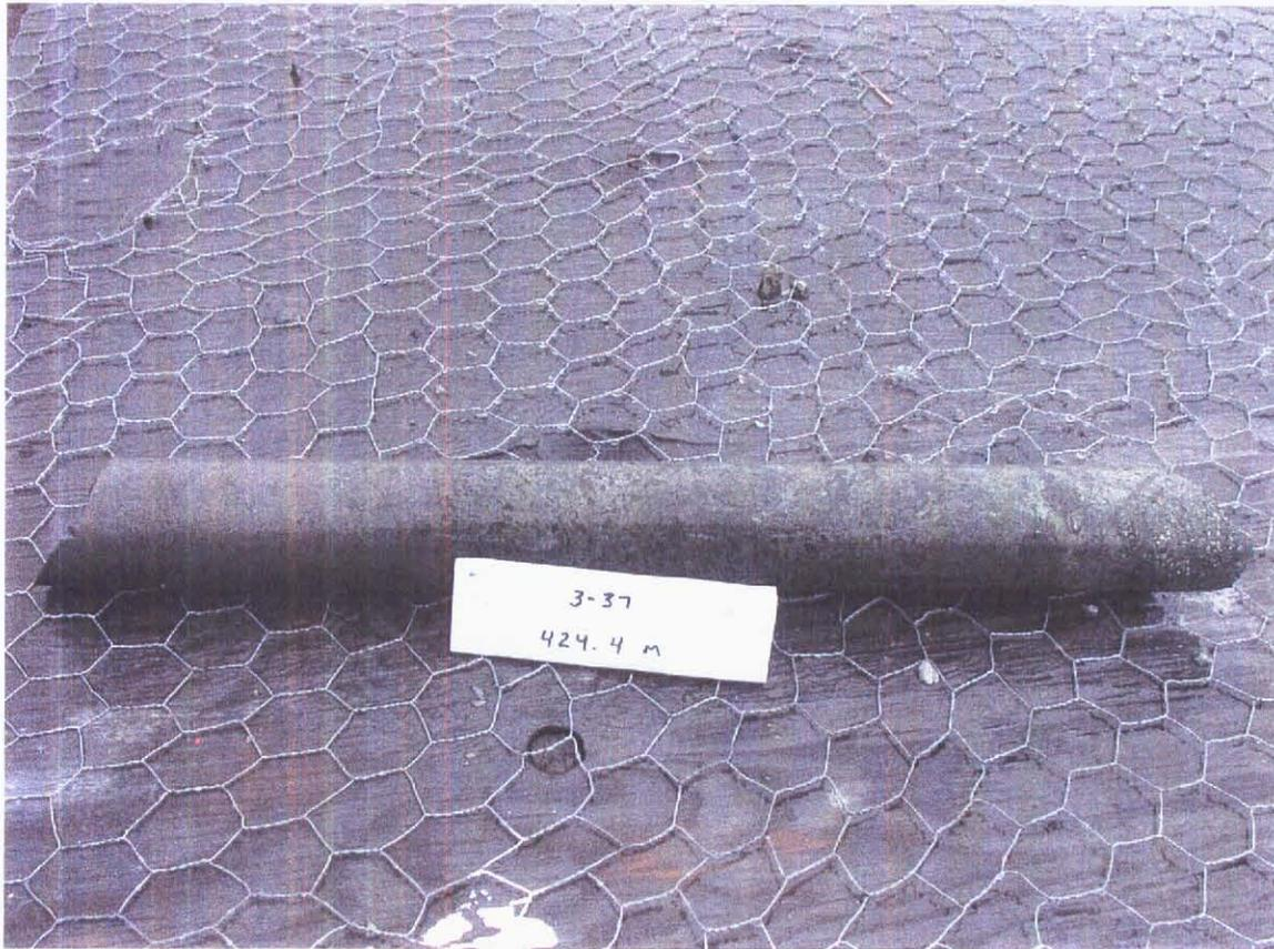
**Plate 6. Chalcopyrite rich calc-silicates, DDH 3 – 37.** This mineralized interval occurs near the footwall contact of the main calc-silicate body with the carbonates, cherts and lesser skarn lenses in the structural footwall of the Canyon Skarn.
