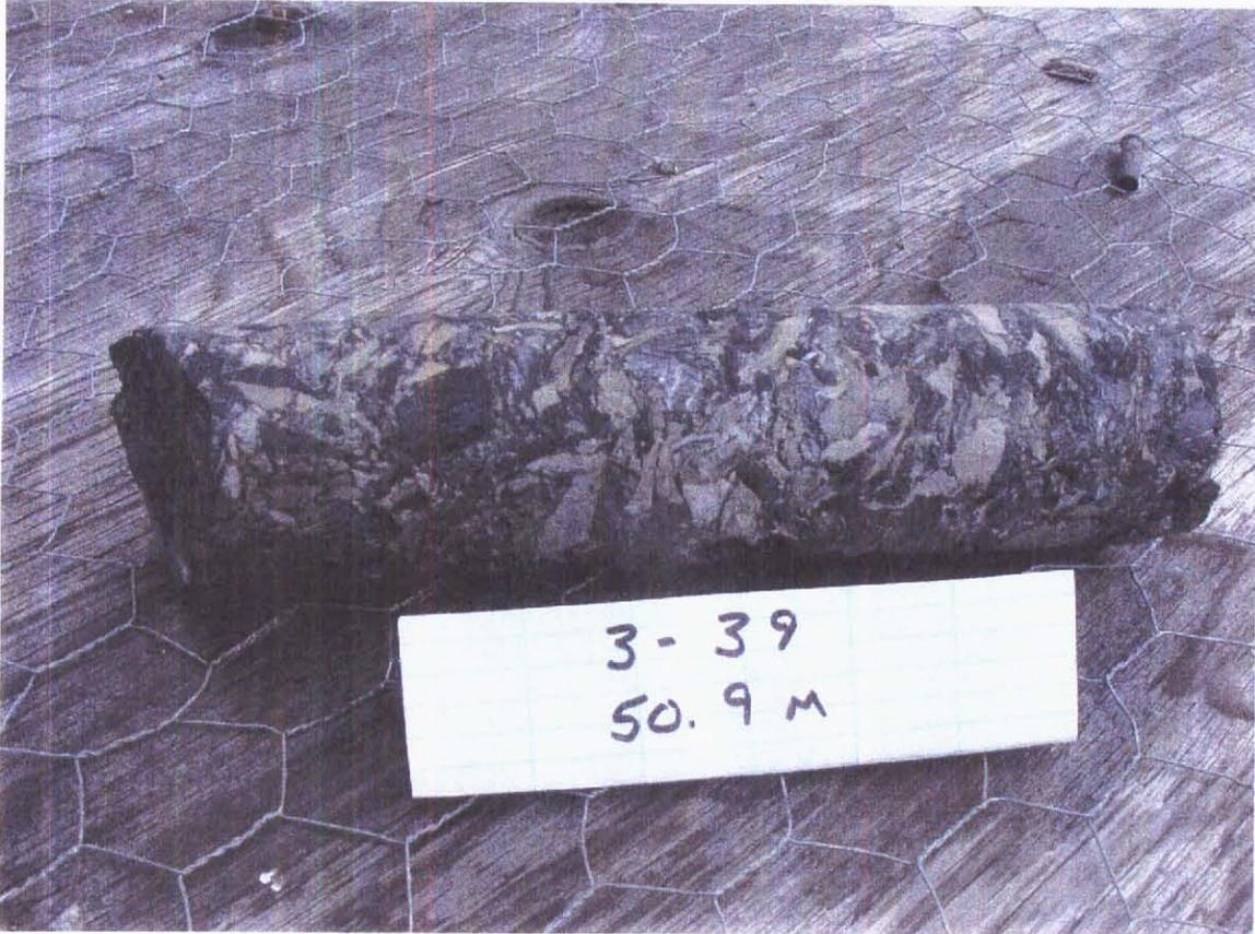
**Plate 8. Angular, depositional breccias, Bralome Takla Mercury mine.** The breccias are likely depositional and not tectonic in origin. No hydrothermal alteration is associated with these breccias and no brittle-ductile fabrics are identified.
