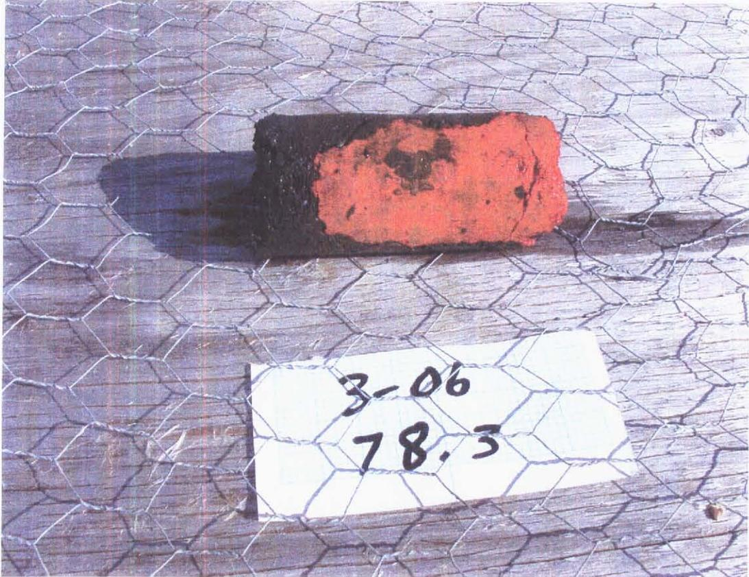
**Plate 2. Coarse cinnabar aggregates cored in DDH 3 – 06.** Significant gold was associated with this interval. Between 77.4 and 78.7 m, 4.46 g/t Au, 1565 g/t Ag, 1.31% Zn and 1.19% Pb was cut. This coarse vein and replacement style of mineralization is in marked contrast to the stockwork style of mineralization cored in DDH 3 – 05 and displayed on Plate 3.
