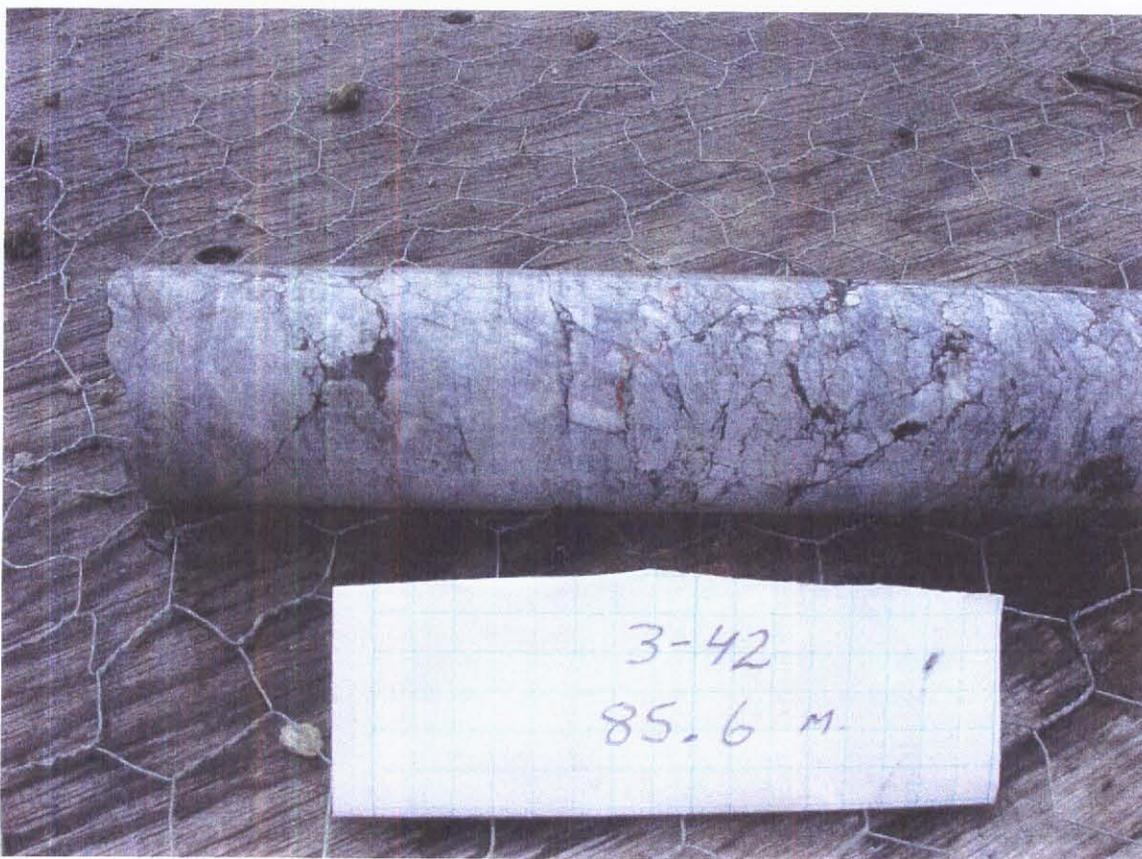
**Plate 9. Distribution of cinnabar in DDH 3 –42.** Small aggregates of bright red cinnabar are noted in the centre of the drill core. No definitive vein association is noted with this mineralized zone.
