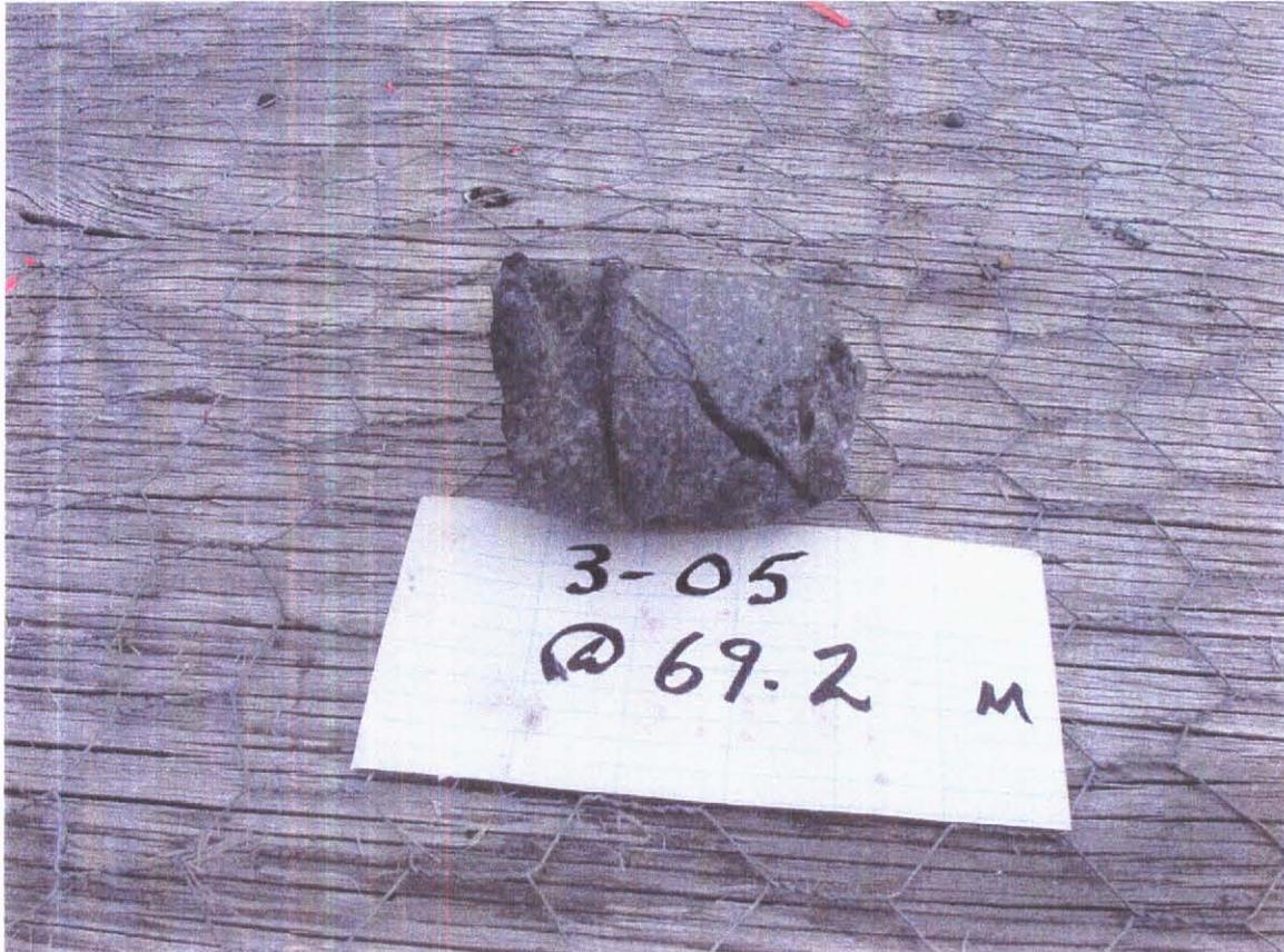
**Plate 3. Stockwork stibnite-silver-gold mineralization DDH 3 – 05.** Mm scale stibnite-silver-lead zinc veinlets and stockworks cut a pale grey-green feldspar porphyritic dyke. The sample is very characteristic of the style and form of mineralization contained within feldspar porphyritic dykes when adjacent to major faults. This interval carried 0.7 g/t Au, 180 g/t Ag, 0.6% Pb and 1.3% Zn.
