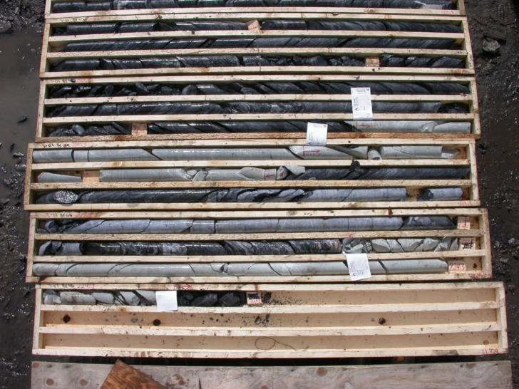
**Diamond Drill Log DDH 3-02**Dip: 45, Azi: 270, T.D.: 151.2 m. North 6160598 +/-10 m, East 347945 +/- 10 m
