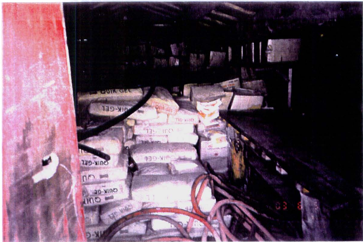
DRILLER'S MUD SUPPLIES IN DRILLER'S BUILDING
