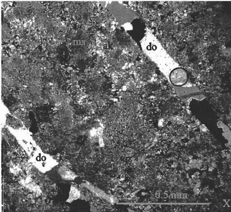
03 IMP04-1 Cryptocrystalline magnesite replaced by slightly coarser grained ankerite and minor patches of quartz; late veinlets of dolomite/magnesite.
