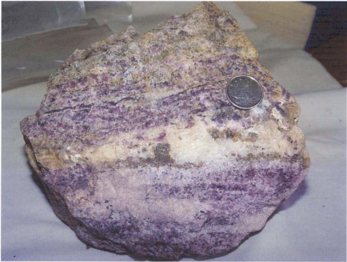
Figure 7 - IR-04-R-02 – Most strongly fluorite mineralized piece of fluoroite-bearing psammite in sample. Fluorite crystals range from lavender to deep purple in colour and from 1 - 10 mm in diameter. Alternating fluoroite-rich and fluorite poor bands define gneissic texture in psammite, with thin, discontinuous bands of sulphides comprised of pyrite ± sphalerite ± galena. Dime for scale.
