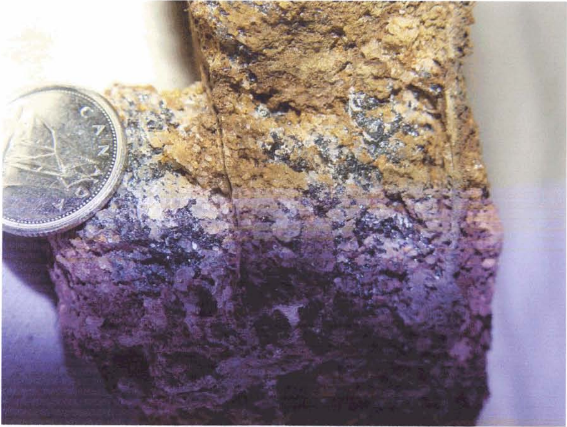
Figure 9 - IR-04-R-04 - Rotten, friable, semi-massive sulphides in psammitic host. Medium-grained, sub-idioblastic sphalerite grains in grain-to-grain contact disseminated in sulphide-rich band up to 4 cm thick, appears to pinch out over 6 cm, may be boudinaged sulphide-rich lozenge. Dime for scale.
