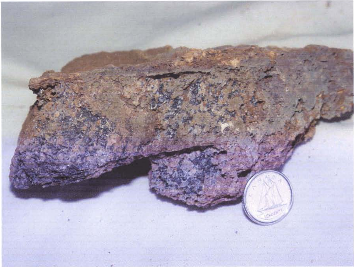
Figure 8 - IR-04-R-03 - Heavily iron-stained, semi-massive to massive sulphides from east end of "E" Zone area. Fine-grained galena \pm sphalerite comprises 70-85% of rock in quartzofeldspathic host. Dime for scale.
