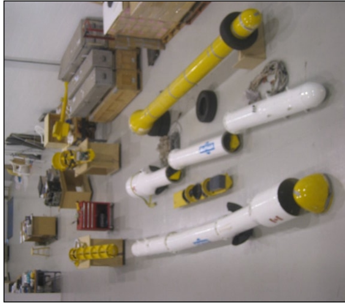
Two 5-frequency and a 4-frequency (in yellow) HUMMINGBIRD sensors undergoing preparations for the field at McPhar's offices in Newmarket, Ontario
