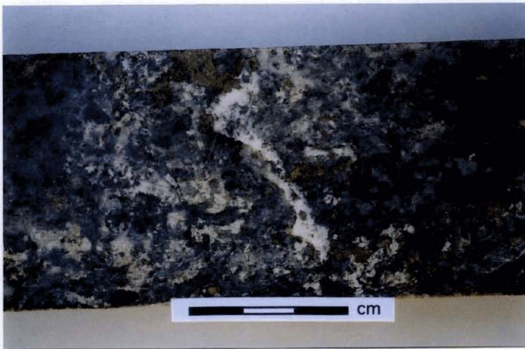
FIG. 19: SAMPLE S91-76, 42.6-42.7m (Macrophotograph of sawn drill core, wet, bar for scale; Film 1 / Frame 9) Strong pervasive alteration has generated moderately abundant scheelite (cream colour, ragged to blocky patches at bottom left, bottom right) with associated aggregates of sulphides (lustrous metallic silvery yellow colour, centre, top centre), abundant K-feldspar (pale greenish cream colour), and calcite (white) filling indistinct fractures (centre).
