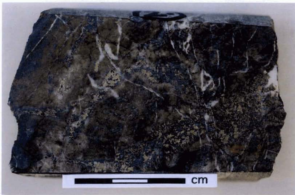
FIG. 6: SAMPLE S91-76, 27.55m (Macro photograph of sawn drill core, wet, bar for scale; Film 3 / Frame 2) Minor late thin discontinuous fractures are filled mainly by calcite (white), and cut hostrock that has suffered strong pervasive alteration by abundant K-feldspar (pale brownish cream) with associated fractures filled by lustrous sulphide (pale metallic silvery colour, centre left, lower right).
