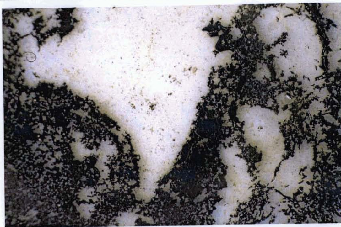
FIG. 3: SAMPLE 91.76/34933 (Macrophotograph of polished thin section, 2.7 cm left to right; Film 1 / Frame 1) This view of part of the polished thin section illustrates the fragmental texture of the rock, emphasised by concentration of arsenopyrite (black grains) in matrix which encloses sericite-K-feldspar altered lithic fragments (colourless).
