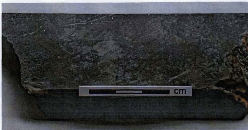
FIG. 2: SAMPLE 91.76/34933. Reverse (unpolished) surface of drill core slice, oblique view. Small grains of native gold (bright metallic yellow) are observable, especially near the thin white fracture at upper left.
