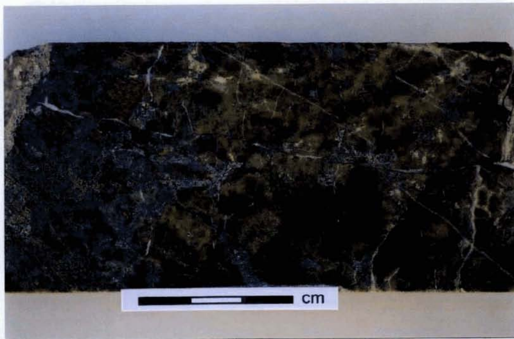
FIG. 15: SAMPLE S91-76, 28.5m (Macro photograph of sawn drill core, wet, bar for scale; Film 1 / Frame 7) Minor late thin fractures (white, filled mainly by calcite) cut hostrock that contains irregularly oriented fractures filled by sulphides (lustrous metallic silvery grey colour, centre left) and associated strong pervasive alteration dominated by K-feldspar (drab paler brownish cream colour).
