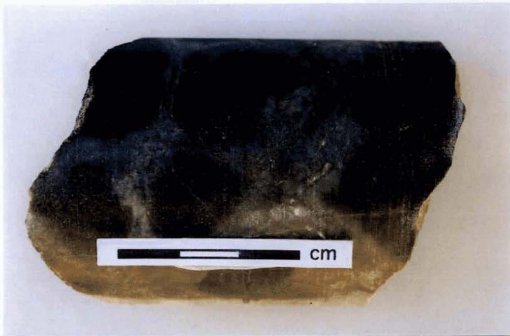
FIG. 26: SAMPLE S91-76, 44.55m (Macrophotograph of drill core, curved surface, wet, bar for scale; Film 1 / Frame 12). This view illustrates intersecting thin fractures (oriented N-S, E-W) sealed by fine-grained lustrous sulphide (metallic silvery colour) and selvaged by K-feldspar (pale greenish cream). Relict dark brownish green hostrock kernels (top left, bottom left, centre, right) contain abundant biotite from a precursor alteration event. Note that the mineralised fracture fillings are very thin, and most of the width of the pale 'veins' is actually alteration selvage.
