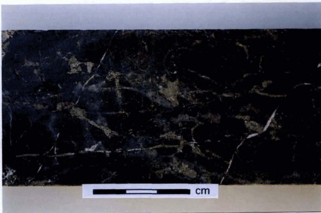
FIG. 16: SAMPLE S91-76, 42.5-42.6m (Macro photograph of sawn drill core, wet, bar for scale; Film 1 / Frame 8) Irregularly oriented and discontinuous fractures are filled mainly by sulphide (lustrous metallic silvery-yellow colour), and are associated with pale greenish cream (K-feldspar-rich) alteration selvages. Relict kernels (dark green) contain abundant biotite from precursor alteration event. Minor late thin fractures are filled by calcite (white).
