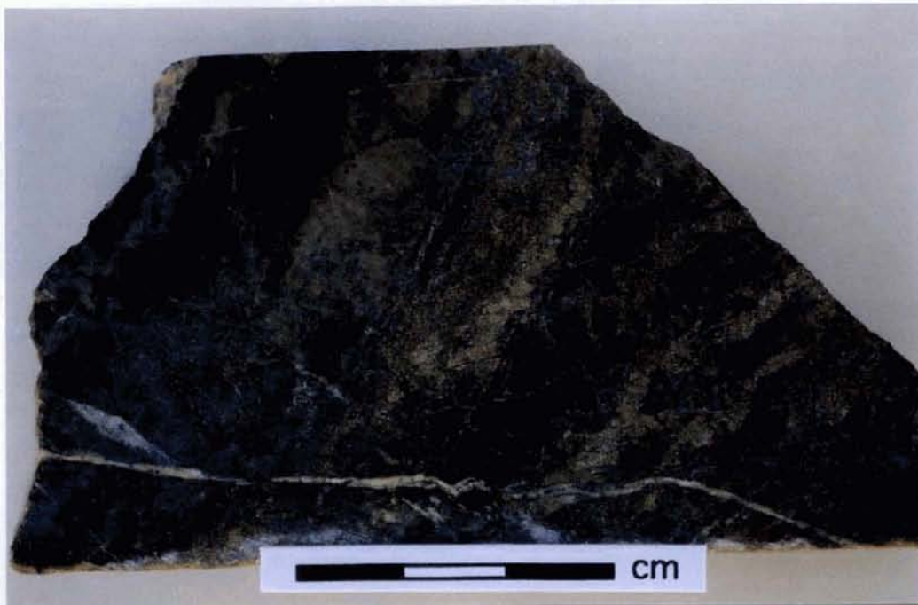
FIG. 8: SAMPLE S91-76, 28.4m (Macrophotograph of sawn drill core, wet, bar for scale; Film 1 / Frame 6) Minor late thin fractures are filled by calcite (white, bottom). The rock has suffered strong pervasive alteration to abundant K-feldspar (pale drab brownish cream to greenish colour) in association with sulphide-filled fractures (oriented NE-SW, near centre and lower right, abundant lustrous silvery sulphide).
