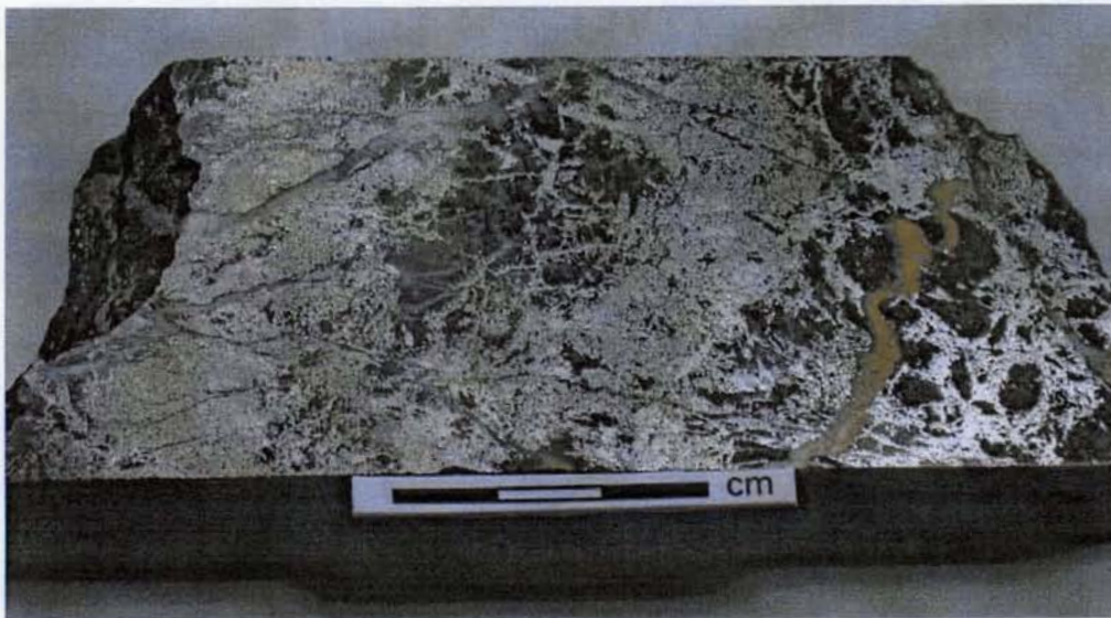
FIG. 1: SAMPLE 91.76/34933. Polished surface of drill core slice, oblique view. Grains of native gold are present, but cannot be discerned in the high lustre of the abundant arsenopyrite (metallic white).
