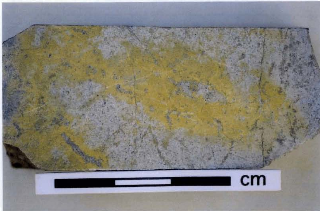
FIG. 1: SAMPLE S91-76, 44.55m (Macrophotograph of section offcut, stained for K-feldspar, dry, bar for scale; Film 3 / Frame 10). This view illustrates lowest intensity of development of K-feldspar (stained yellow) in diffuse selvages marginal to thin indistinct sulphidic fractures (oriented NE-SW, at bottom left, and across centre). Relict kernels of precursor rock (bottom, top right) contain much biotite from the earlier potassic alteration assemblage.
