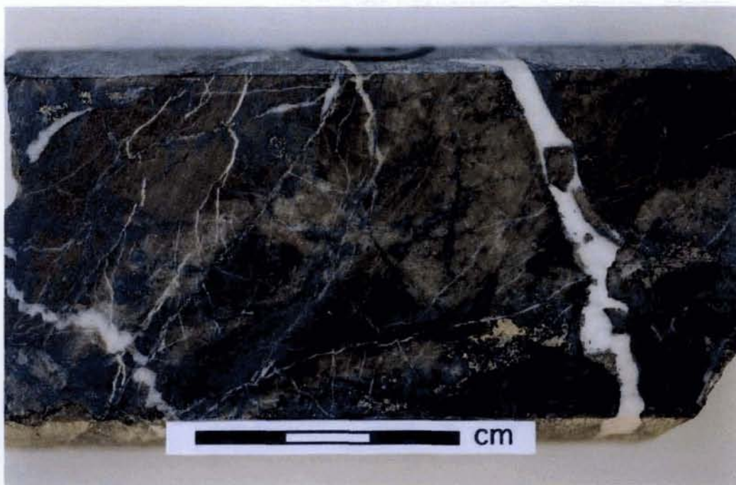
FIG. 3: SAMPLE S91-76, 27.4m (Macrophotograph of sawn drill core, wet, bar for scale; Film 3 / Frame 1) Late brittle fractures (white) are filled mainly by calcite, with minor sulphides (marcasite, sphalerite) along some fracture filling margins (left margin of fracture filling at lower right). Dark patches represent relict kernels of precursor biotite-altered hostrock, overprinted by the paler K-feldspar-rich assemblage.
