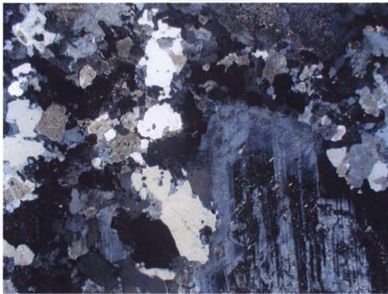
SND 372 @241: Representative views showing fine-grained subhedral granular quartz, K-feldspar and plagioclase. A large plagioclase phenocryst is present on the right side of photo B. A) PPL, B) XPL, FOV = 6 mm.
