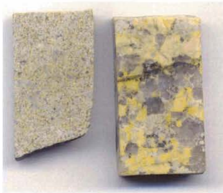
Sample 372 @ 241 (left) and SND 386 @ 10.3 (right), showing distribution of K-feldspar (yellow stain) and variation in grain size. Chips are approximately 2.6 by 4.6 cm in size.
