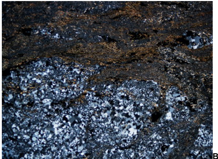
Hen 941 – 69.5: Representative view showing bands of quartz , biotite, K-feldspar and sulfides FOV = 8.5 mm, A) PPL, B) XPL
