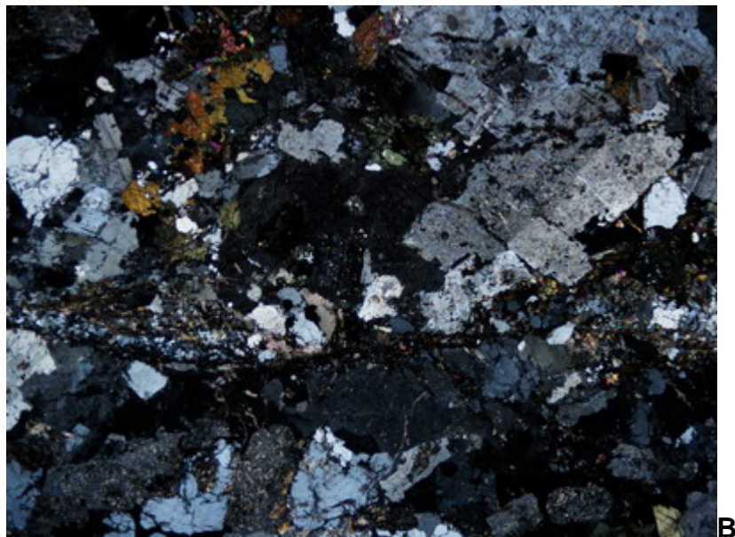
SB DDH3 -130: Representative view showing plagioclase, orthoclase, minor quartz and hornblende replaced by chlorite and epidote. FOV = 8.5 mm, A) PPL, B) XPL
