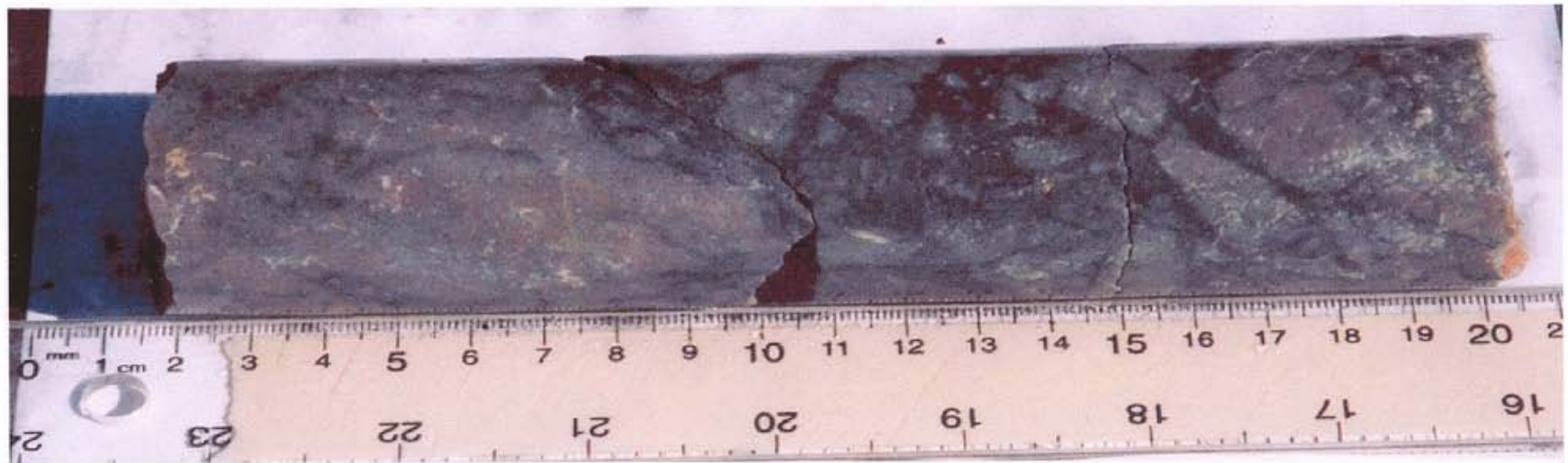
PHOTO 26: DDHSZD04-01: SULFIDE MATRIX QUARTZ BRECCIA VEIN. SAMPLE 599601: 3.41 g/Au/t, 991 ppm Au, 346 ppm As over 0.5 m (102.27 - 102.77 m).
