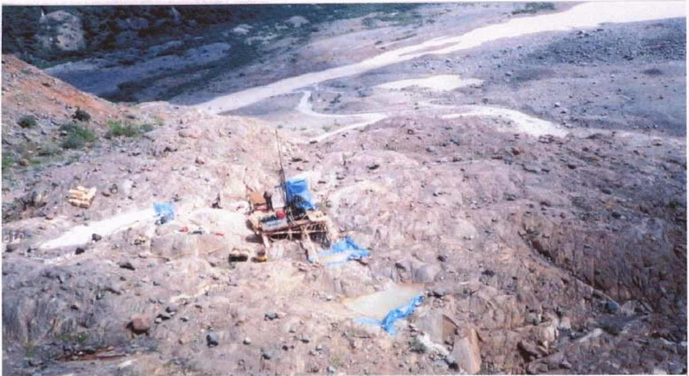
PHOTO 8: DDHSZD04-04: LOOKING SOUTHEAST ON DRILL SET-UP AND FOUR SUMP PONDS USED FOR DDHSZD04-01, 02A, 03 AND 04. NOTE CLEAR WATER IN LOWEST POND. TODD CREEK VALLEY IS IN BACK GROUND.
