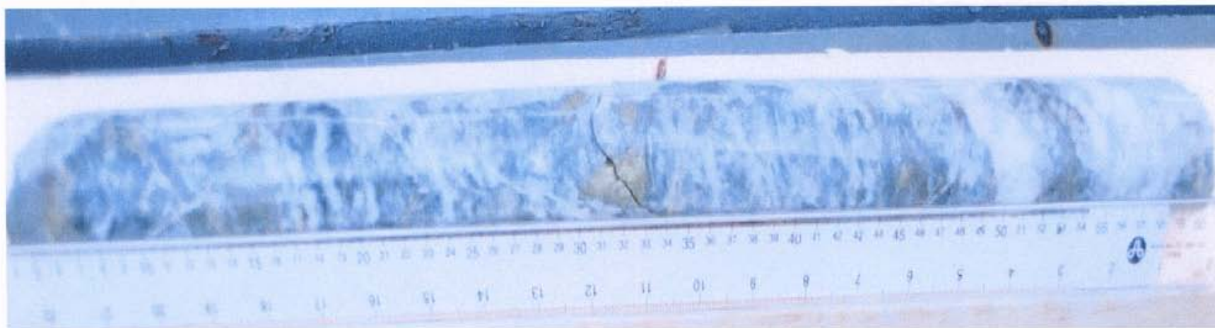
PHOTO 32: DDHSZD04-02A: QUARTZ-HEMATITE-SULFIDE VEIN (M TYPE MINERALIZATION) BRECCIA VEIN, SZDS. SAMPLE 609754: 10.29 g Au/t, 1.34% Cu over 0.9 m.
