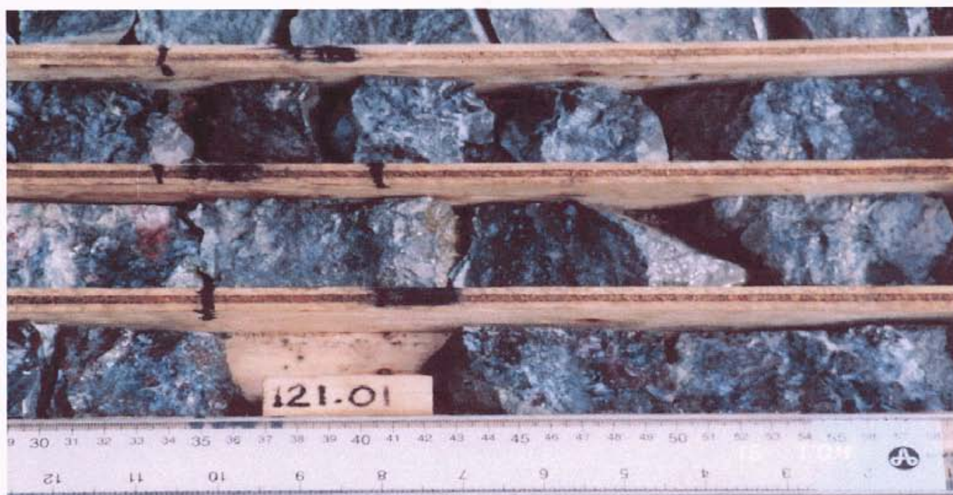
PHOTO 24: NEXT04-01 @ 121.01 m, BOX 28: HEMATITE-BLEBBY CHALCOPYRITE QUARTZ BRECCIA VEIN. SAMPLE 609151: 1.55 g Au/t, 0.49% Cu, 631 ppm As.
