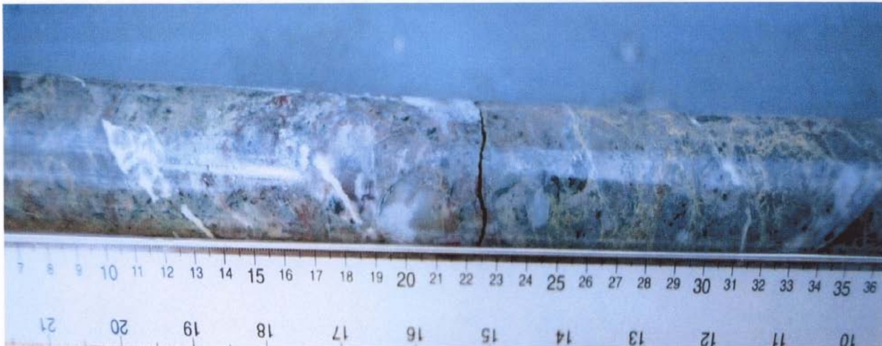
PHOTO 31: DDHSZD04-02A: QUARTZ-HEMATITE-ANKERITE MULTIPHASE BRECCIA VEINS, SZDS. SAMPLE 609753: 0.09 g Au/t, 0.11% Cu over 1.12 m.
