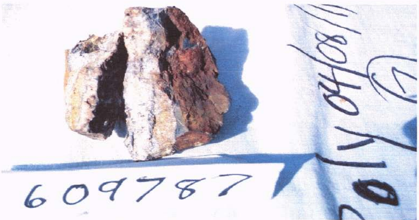
PHOTO 4: SAMPLE 609787RF - TYPE 1 MINERALIZATION: QTZ-SULFIDE VEIN IN ANGULAR ROCK FLOAT AT STN 380 M N ON HWY ZONE CRK CONTROL LINE: 40.5 PPM AU, 812.3 PPM AG, 8745 PPM CU, 1652 PPM PB, 1703 PPM ZN, 645 PPM AS, 209 PPM SB, 21.7 PPM SB (WITH RESULTS OF 2 AU & 2 AG ANALYSES AVERAGED).
