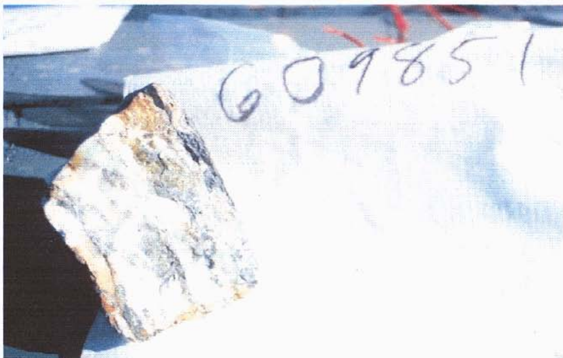
PHOTO 14: ROCK FLOAT SAMPLE 609851RF OF TYPE 1 QUARTZ-SULFIDE VEIN MATERIAL TAKEN OVER IP ZONE C ON THE MC CL AT L56N: 3.11 G AU/T (BASED ON THE AVERAGE OF 2 GOLD ASSAYS), 37.5 G AG/T, 0.04% CU, 0.03% PB AND 0.03% ZN.
