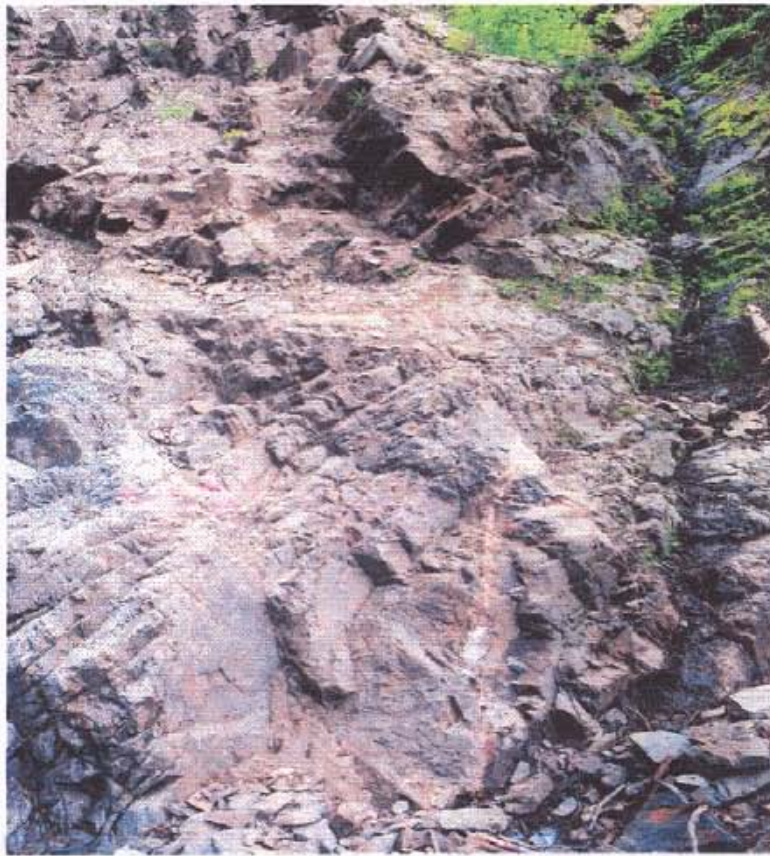
PHOTO 11: 429 VEIN AT 60+29N ON HZC CL. AREA OF SAMPLES 609869R AND 609870R WITH TYPE 1 QTZ-SULFIDE MINERALIZATION: 6.44 G AU/T (BASED ON THE AVERAGE OF 2 GOLD ASSAYS), 48.5 G AG/T, 0.05% CU, 0.05% PB AND 0.72% ZN; AND, 7.43 G AU/T (BASED ON THE AVERAGE OF 2 GOLD ASSAYS), 75.10 G AG/T, 0.08 PPM CU, 0.04 PPM PB AND 0.03 PPM ZN, RESPECTIVELY.
