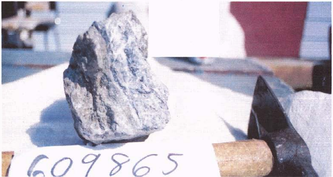
PHOTO 5: SAMPLE 609865RF - QTZ-CARB-SULFIDE BRECCIA VEIN IN ROCK FLOAT AT 380 M N ON HWY ZONE CRK CONTROL LINE: 16 PPM AU, 222.9 PPM AG (WITH 2 AU & 2 AG ANALYSES AVERAGED), 2208 PPM CU, 560 PPM PB, 986 PPM ZN, 485 PPM AS, 35 PPM SB, 2.4 PPM CD. THE SAMPLE & THE SAMPLE SHOWN BELOW (609787RF) ARE THOUGHT TO HAVE COME FROM THE AREA OF THE HISTORIC HWY ZONE CREEK SHOWING (~380 - 430 M N).
