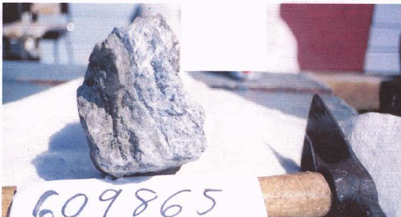
PHOTO 5: SAMPLE 609865RF - TYPE 1 MINERALIZATION: QTZ-CARB-SULFIDE BRECCIA VEIN IN ANGULAR ROCK FLOAT AT STN 380 M N ON HWY ZONE CRK CONTROL LINE: 16 PPM AU, 222.9 PPM AG, 2208 PPM CU, 560 PPM PB, 986 PPM ZN, 485 PPM AS, 35 PPM SB, 2.4 PPM CD (WITH RESULTS OF 2 AU & 2 AG ANALYSES AVERAGED). THE SAMPLE & THE SAMPLE SHOWN BELOW (609787RF) ARE THOUGHT TO HAVE COME FROM THE AREA OF THE HISTORIC HWY ZONE CREEK SHOWINGS (~380 - 430 M N).
