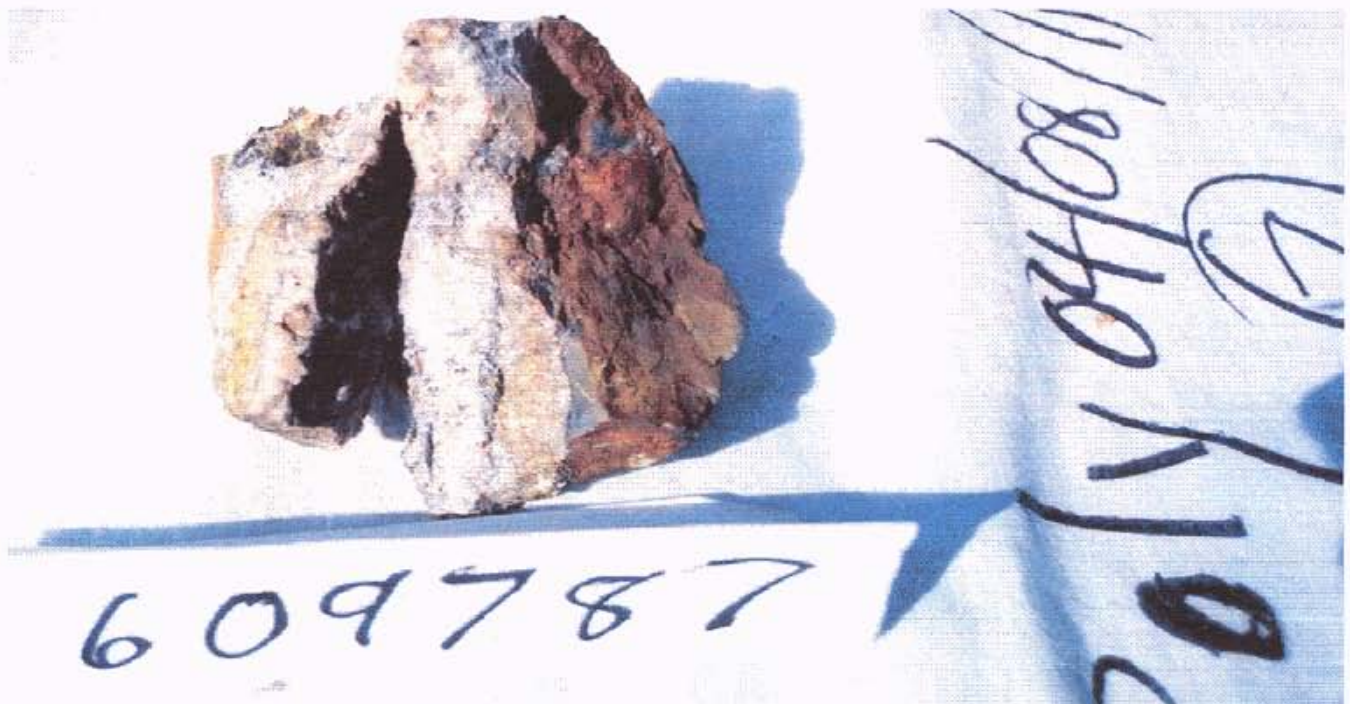
PHOTO 4: SAMPLE 609787RF - QTZ-SULFIDE VEIN IN ANGULAR ROCK FLOAT AT STN 380 M N ON HWY ZONE CRK CONTROL LINE: 40.5 PPM AU, 812.3 PPM AG (WITH 2 AU & 2 AG ANALYSES AVERAGED), 8745 PPM CU, 1652 PPM PB, 1703 PPM ZN, 645 PPM AS, 109 PPM SB, 21.7 PPM CD .
