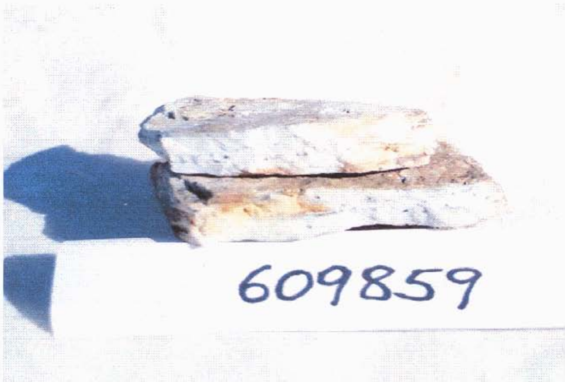
PHOTO 13: ROCK FLOAT SAMPLE 609859RF AT 58+35N ON THE HZC CL WITH TYPE 1 MINERALIZATION IN QUARTZ-COARSE SULFIDE VEIN MATERIAL: 4.01 G AU/T, 49.90 G AG/T, 0.04% CU, 0.30% PB, AND 0.39% ZN.
