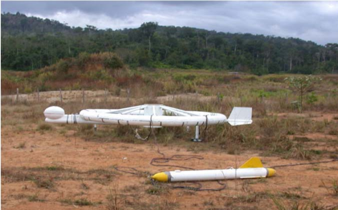
Figure 3: The magnetometer bird (foreground) and AeroTEM II EM bird
