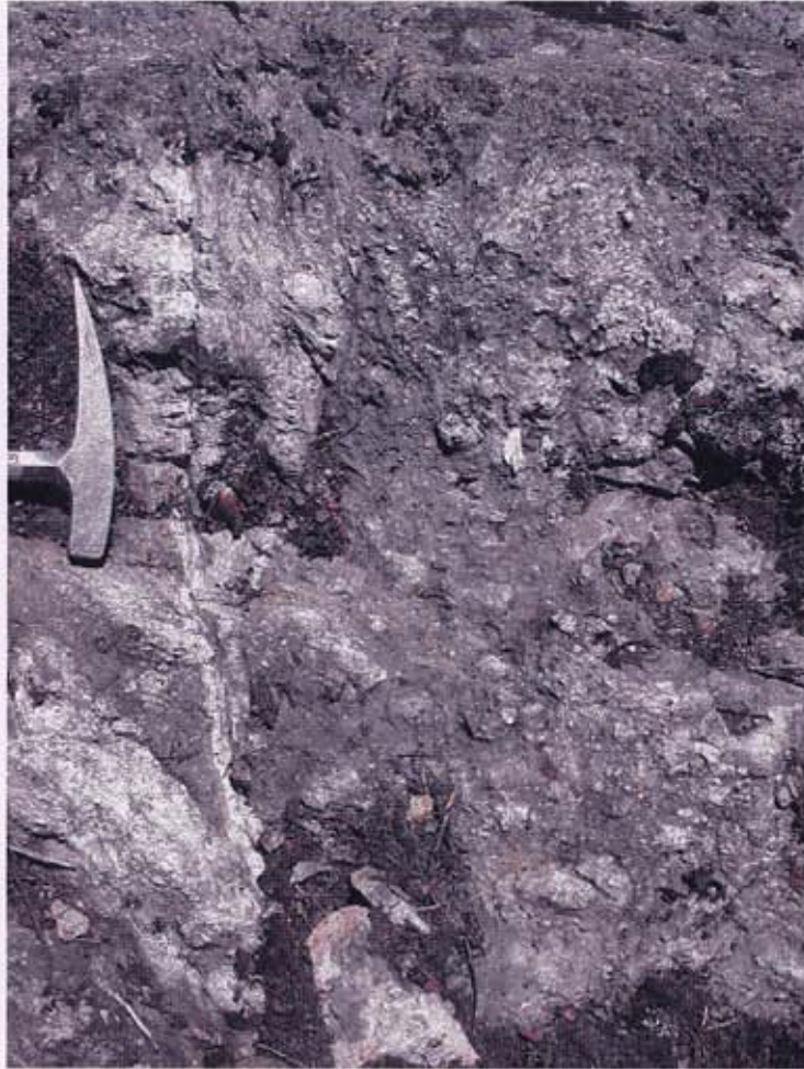
Photo 2826; station KD 27-23: Shear zone with gouge and subangular to subrounded breccia fragments in a very fine-grained matrix. FOV ~ 50cm
