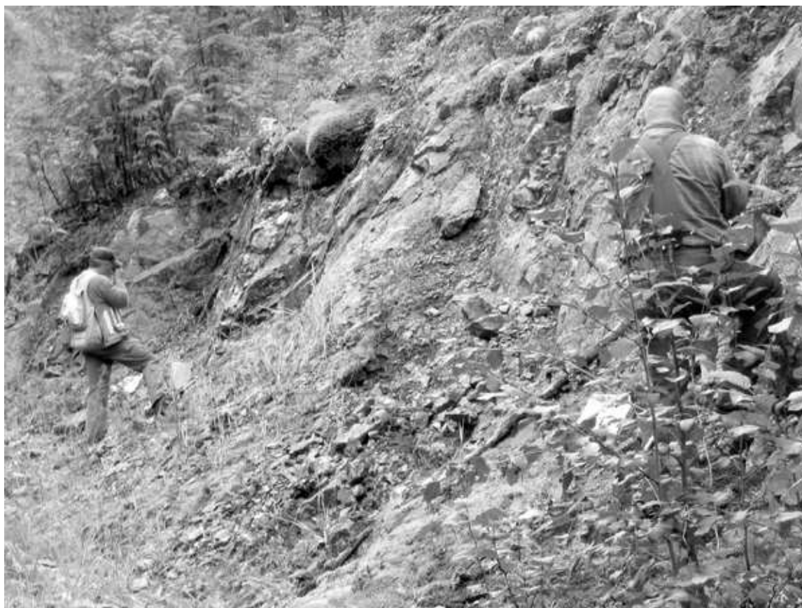
Fig. 15 C. Kennedy (foreground) & B. Doyle examining Limpid Roadside Veining in a roadcut along the Limpid Ck Forest Service Road (fig. 3). Quartz veins are intrusion-hosted in the Bunker Hill Sill. Vein orientation 117° 72° SW near parallels the road. Year 2003 samples BH10 & BH11 are anomalous at 594 & 96 ppb gold. In Sept. 2004 0417 0418 & 0419 were sampled. 0417 has anomalous Au 0.13 / Ag 1.3 / Mo 490 / Pb 375 / As 98, all ppm. Bi and Te are background. Some vein fractures are tourmaline-coated. The site is 650 m N of BiTel Knoll veins along the same W contact of the Bunker Hill Sill.
