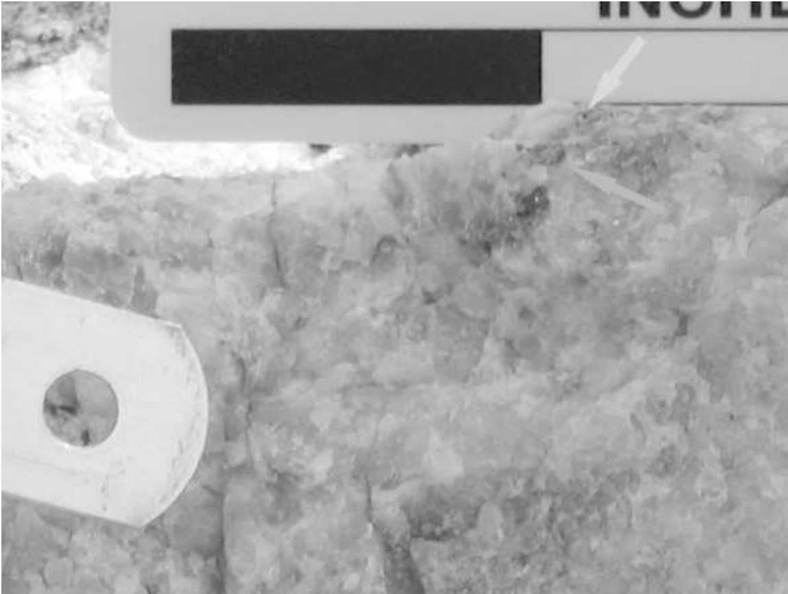
Fig. 10 Close-up of previous photo, site of grab sample 0515 of angular float from Eloise Vein North. Top arrow marks a coarse gold grain. Bottom arrow marks a clot of coarse sized bismuth minerals with several flecks of fine-grained gold. The bismuth mineral is likely bismuthinite. Both may be decomposition products from sulfidation of early maldonite. Quartz has a v light grey cast in the photo – card is actually white and tag steel-grey. Limonite-coated fractures trend about the same as the Bi + Au clot.
