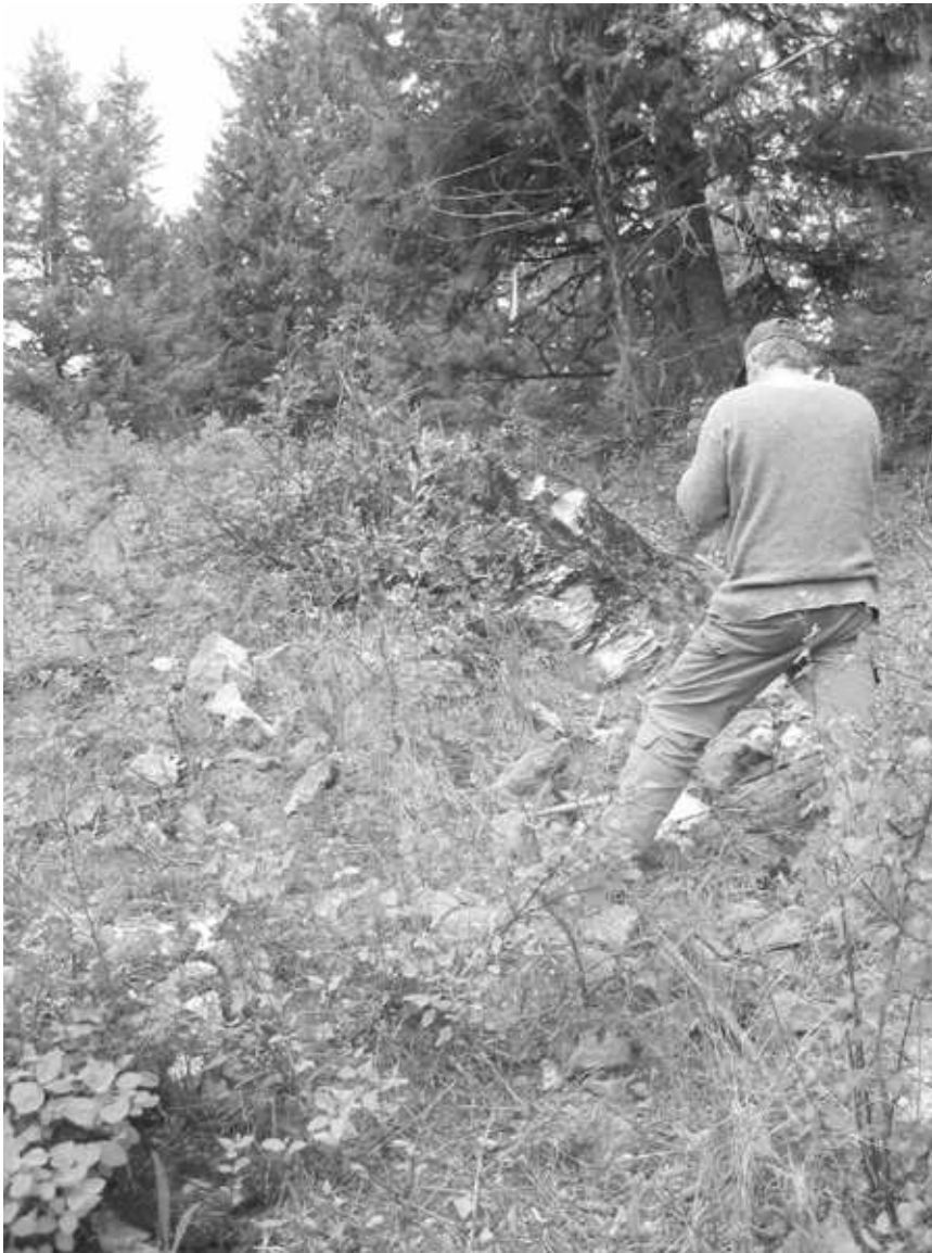
Fig. 8 B. Doyle further uphill on resistant Eloise Vein South. View to NNE. A 30 cm chip sample 0517, with W-E oriented 'pages-of-a-book' fracturing above left knee, ran 2.76 g/t Au by fire assay. Several sub-mm sized, very fine-grained native gold specks were observed on collecting the sample, all near limonitized patches.
