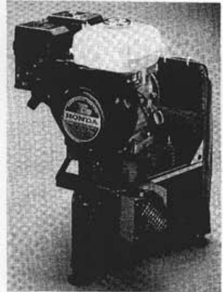
**MG - 2 :** 2KVA motor generator. This versatile unit is adequate for the vast majority of IP and resistivity surveys conducted worldwide. It is light enough to be carried by one man, yet powerful enough for most survey requirements. The motor is a 4-cycle Honda which produces 5 HP at 3600 rpm. The dimensions of the unit, including packframe, are 40 x 45 x 60 cm (16 x 18 x 24 in). Total weight is 34 kg (75 lb.).
