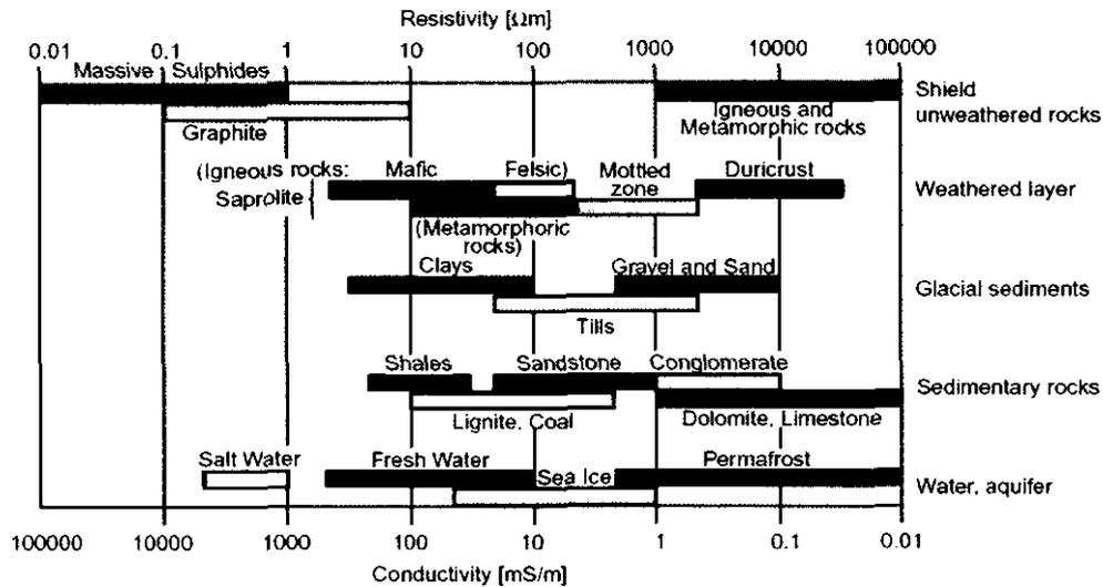
Figure 3: The resistivity (reciprocal of electrical conductivity) range of some geological materials.
