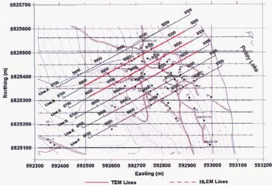
Figure 1b: TEM and HLEM line locations in the Wishbone area
