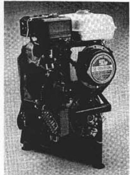
**MG - 3 :** 3KVA motor generator. This two-man portable unit is designed for surveys in areas which require additional power. The motor is a 4-cycle Briggs and Stratton which produces 8 HP at 3600 rpm. The unit is mounted in a square frame with dimensions 40 x 48 x 75 cm (16 x 19 x 29 in). Total weight is 55 kg (120 lb.).
