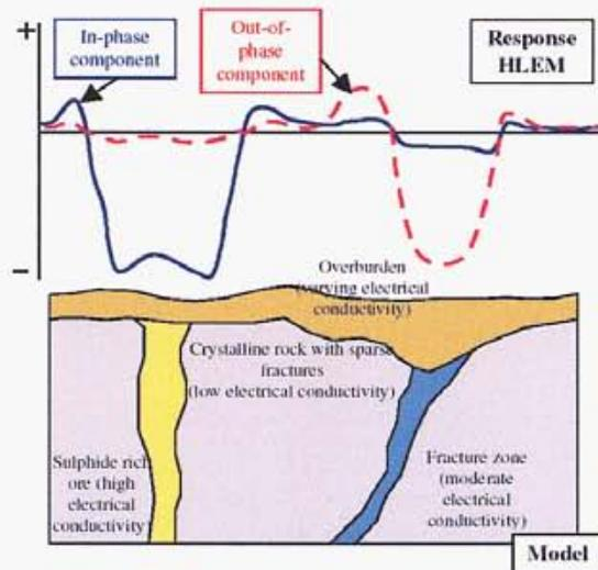
Figure 5: Typical response curves from an HLEM survey.
