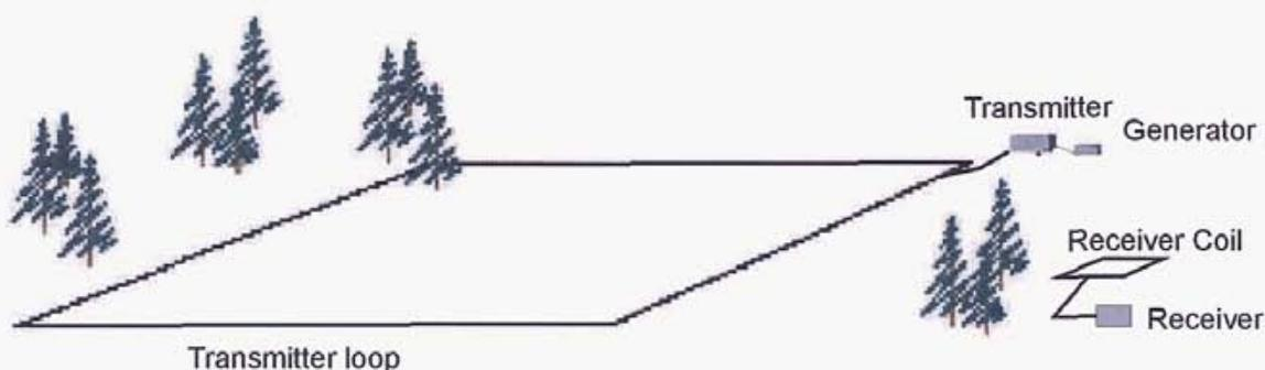
Figure 2: TEM Profiling Configuration
