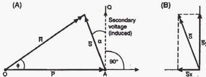
Figure 4: Illustration of the primary and secondary magnetic fields in the HLEM method
