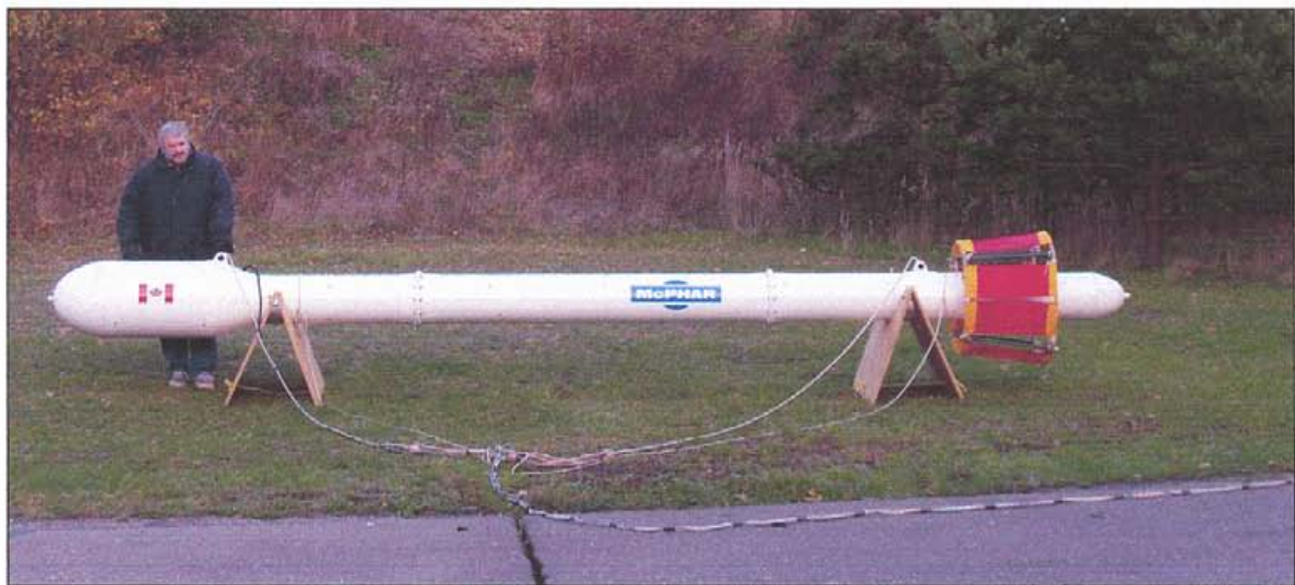
Figure 9: HUMMINGBIRD™ Electromagnetic Sensor
