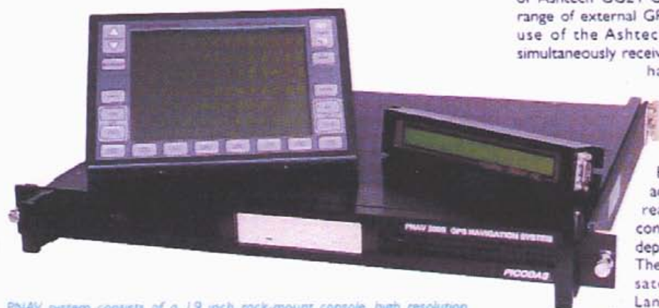
PNAV system consists of a 19 inch rack-mount console, high resolution Moving Map Display with keypad for all system controls and Pilot Indicator display for cross-track guidance.
