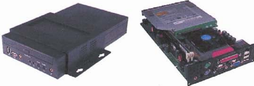
Figures 2 & 3: "mini-footprint" Pentium III computer module
