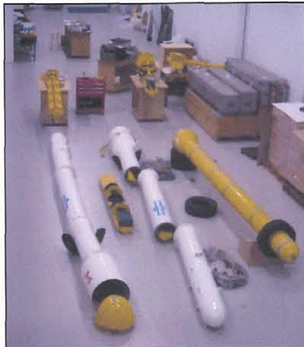
Two 5-frequency and a 4-frequency (in yellow) HUMMINGBIRD sensors undergoing preparations for the field at McPhar's offices in Newmarket, Ontario
