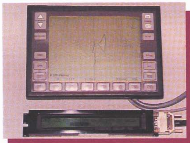
The Moving Map Display and Pilot Indicator can be operated up to 5 m (15 ft.) away from the PNAV console mounted in the operator's or pilot's best view and access. The on-going flight path with overlay of the survey area, flight lines, locked (surveyed) line and waypoints, ground speed, heading, cross-track information and distance-to-go are calculated and displayed in real time on the Moving Map Display, the Pilot Indicator displays all essential navigation and cross-track information.
